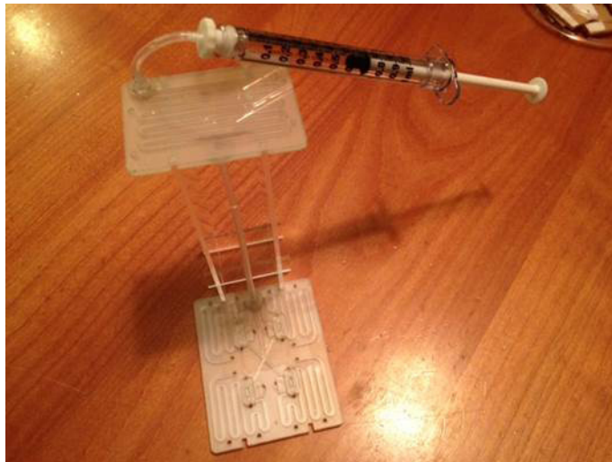
The Biomimetic Lung Toxicity Screening Platform (bioMIMIC) is a practical in-vitro tissue-on-a-chip screening platform that models the air sac/blood vessel interface and is suitable for use in BSL3/4 labs (Project 151350).
