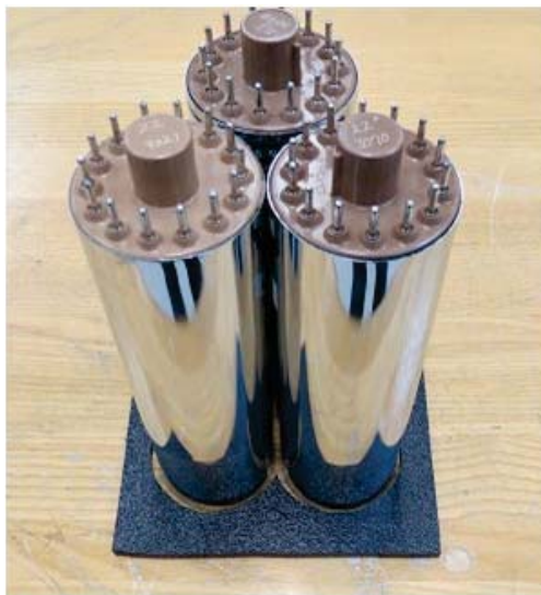
Figure 2. Three NaI:Tl crystals ( 50.8 \times 50.8 mm) sit vertically with crystals facing the table. The combination of check sources were moved on the arc of a 50.8 cm radius around the center, and data were obtained in long dwell mode (10 minutes at each angle) to calculate gamma count rate from individual crystals and a summed spectrum; individual amplifier gains were matched before the data run.
