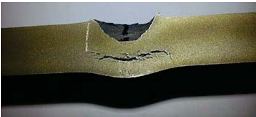
Figure 6. A sectioned target (Test ID 1000-016) plate confirmed spall fracture had occurred
