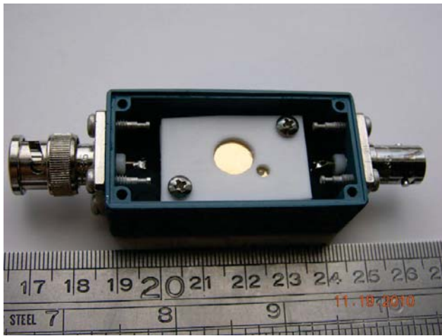
Figure 2. CZT mounted in a Pomona shielded box
