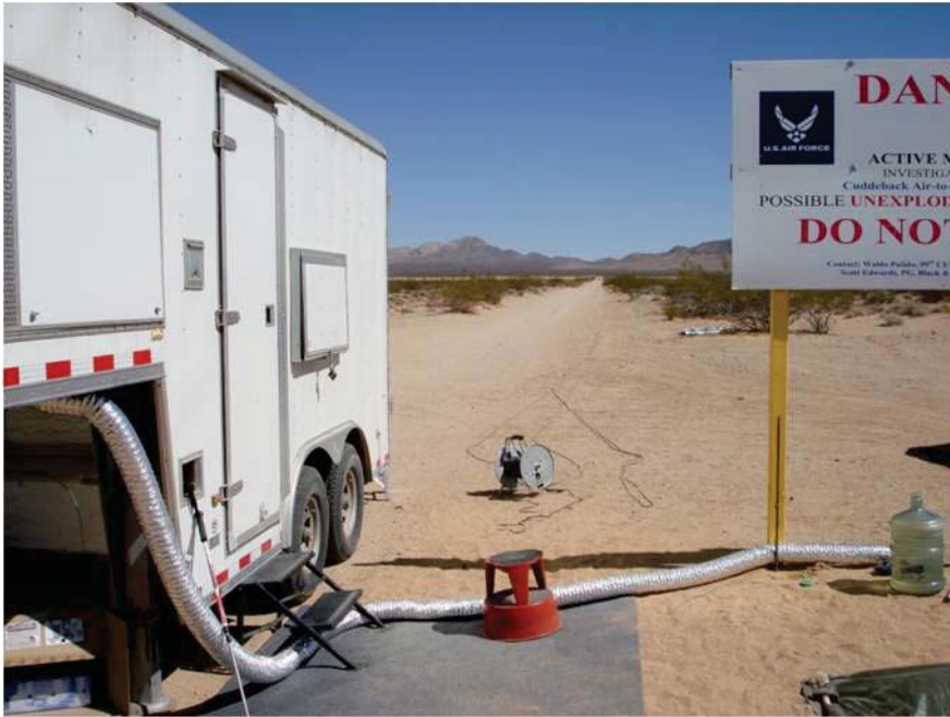
Figure 1. Trailer-mounted system stationed in the Mojave Desert. The small "dot" near the end of the road in the distance is a flatbed truck with one of the 48" square targets at 1 km.
