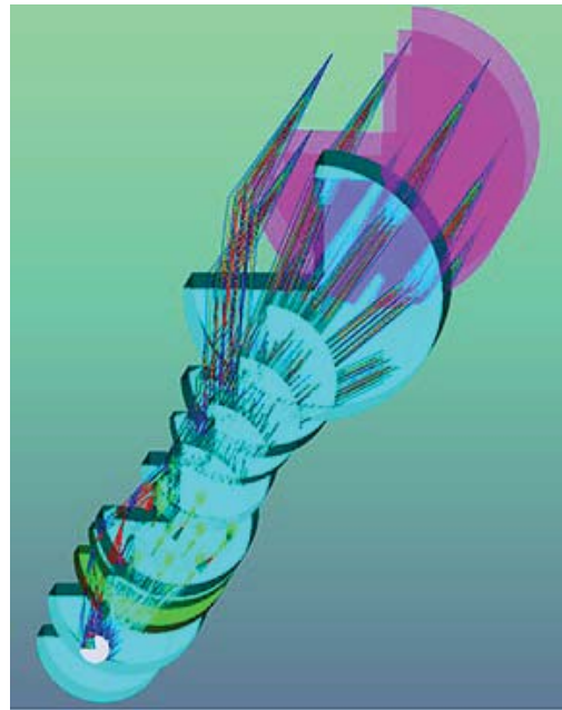
An illustration of the hyperchromatic lens, shown producing images at varying locations as a function of time
