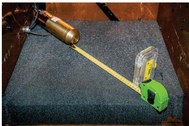
Figure 9. CLYC detector, source, and CLYC detector geometry
