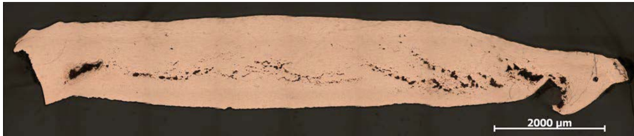
Figure 12. Cross section of the PBX 9501/copper sample showing clear evidence of damage. The feature at the right end is not seen in the radiograph and therefore was likely caused during the recovery process.
