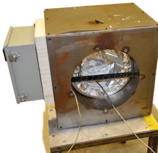
Figure 1. NRS sample oven, shown with the aluminum foil removed on the front, exposing the heating element inside
