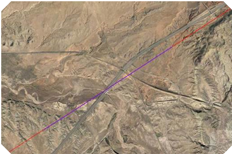
Test flight path, with 3.2 km measurement tail (in purple).
