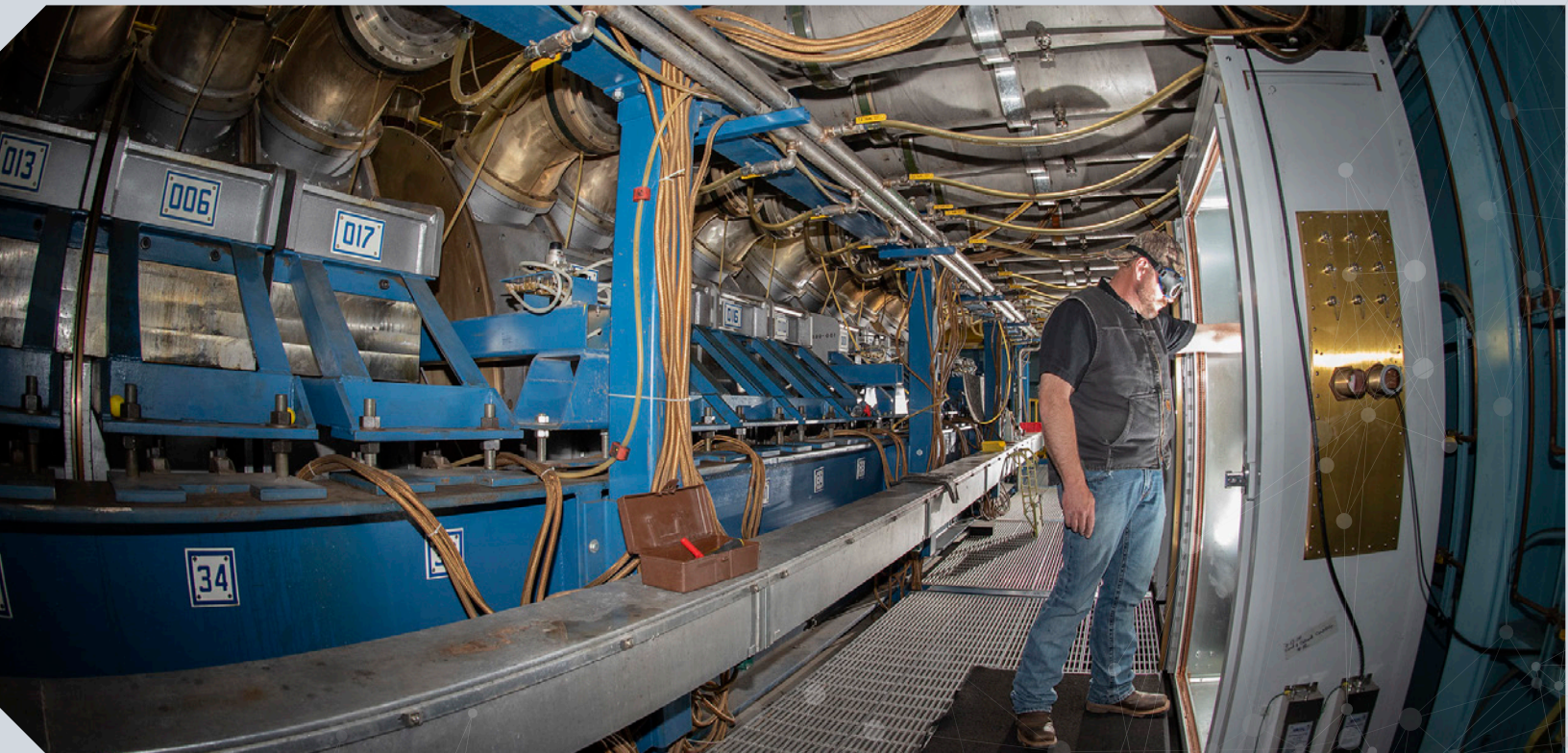
PI Theodore Grabowski led a significant LDRD project in FY20 that utilized the Hermes III accelerator, the world's largest gamma radiation simulator. In this image, one of Sandia's technicians arms a series of triggering lasers for a test.
