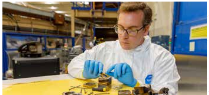
Physicist Chad McCoy at Sandia's Z machine loads sample coatings into holders. When Z fires, researchers will observe how well particular coatings protect objects stacked behind them. (Photo by Bret Latter)
