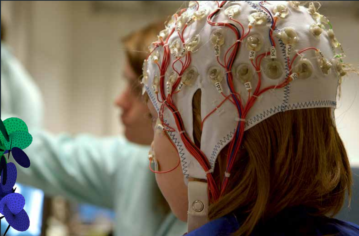
Sandia researchers wore caps like this one outfitted with EEG sensors while participating in an experiment that measures brain activity.
