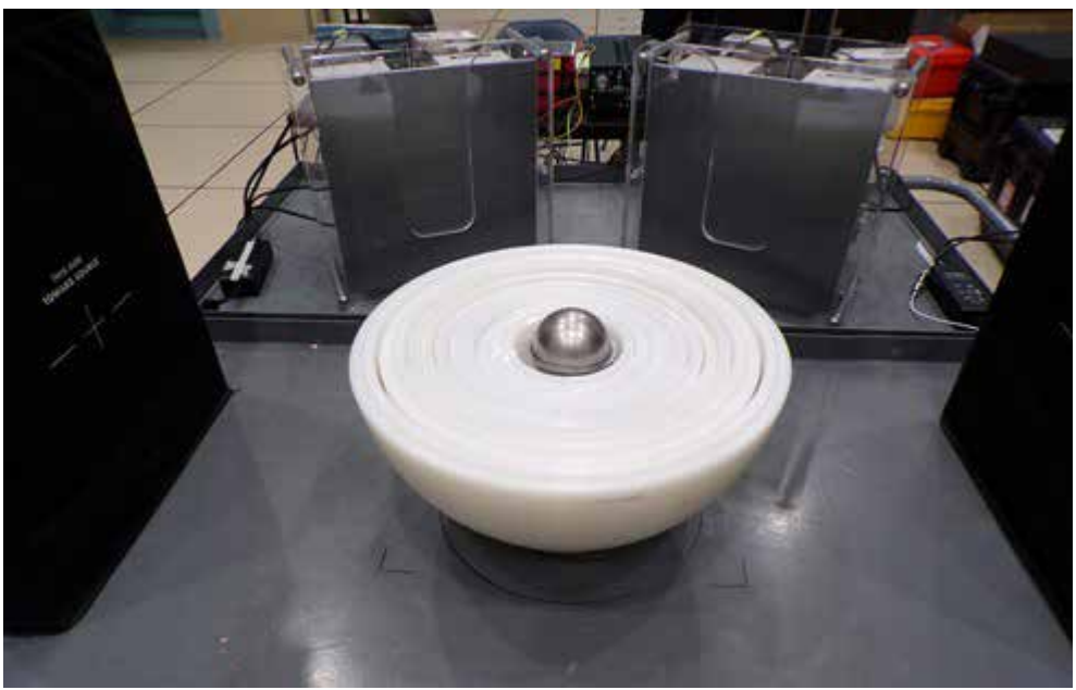
Measurement of a 4.5 kg sphere of weapons grade plutonium moderated by 6" of high-density polyethylene (HDPE) using an array of sodium iodide detectors (rear). In this photo, the moderating sphere is half assembled, which allows the plutonium and the nested HDPE shells to be seen. The measurements were performed using a fully assembled moderating sphere. The nested shells made it possible to assess the performance of the technique using a parametric study over a range of HDPE thicknesses.
