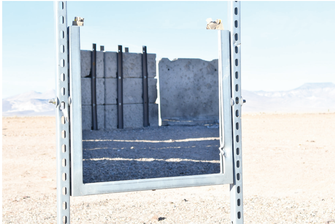
■ Cameras at Kappa West frequently capture experiments reflected in mirrors, which allows the cameras to record safely while avoiding direct exposure to detonations.
