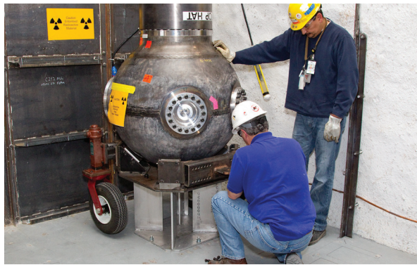
■ Technicians prepare a 3-foot vessel for the Barolo test series, which was executed in the Cygnus test bed in 2011.
