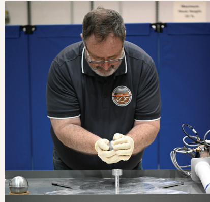
■ Haynes holds a beryllium-reflected plutonium (BeRP) ball at NCERC.
