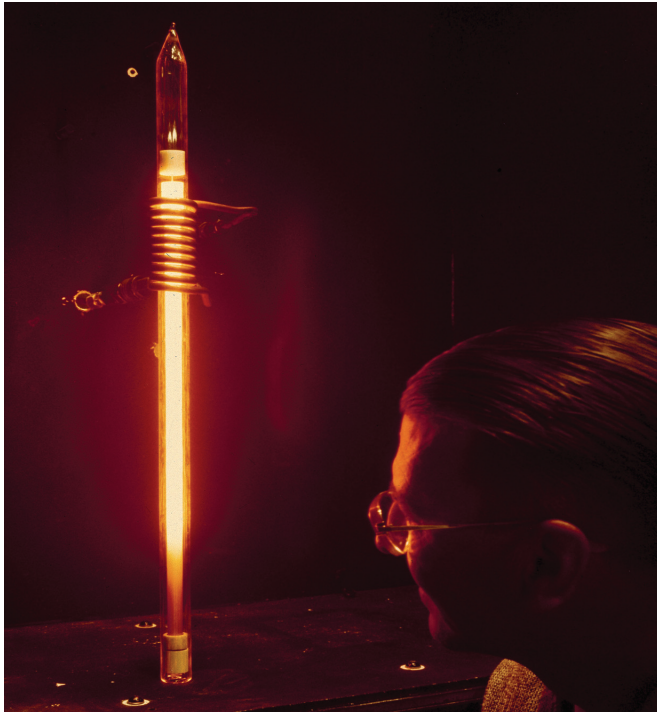
In this photo taken in the early 1960s, physicist George Grover tests a heat pipe.
