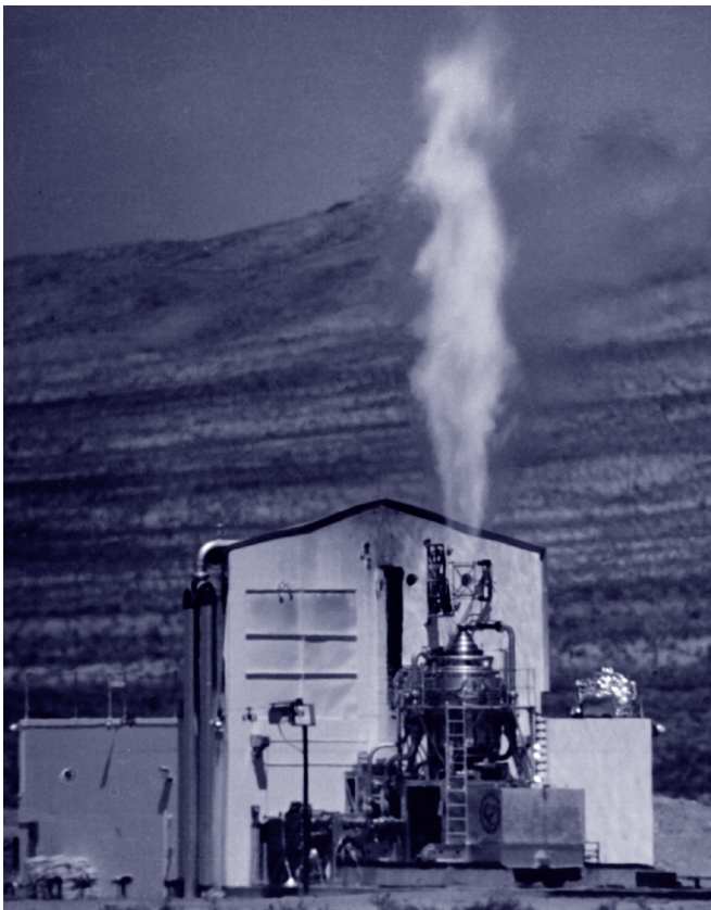
Fig. 4. The Kiwi-A is test-fired, making it the world's first nuclear-rocket reactor to undergo such testing. This image shows an incandescent plume of hot hydrogen gas exiting the reactor's rocket nozzle.
