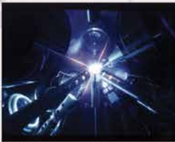
■ Inside the Omega laser's target facility at the moment of operation. Omega is a 60-beam system capable of delivering 30 kilojoules of energy to a target.
