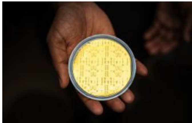
More than a thousand experimental lasers and amplifiers adorn a three-inch, gold-electroplated silicon wafer made at Sandia's Microsystems Engineering, Science and Applications complex. (Photo by Craig Fritz.)
