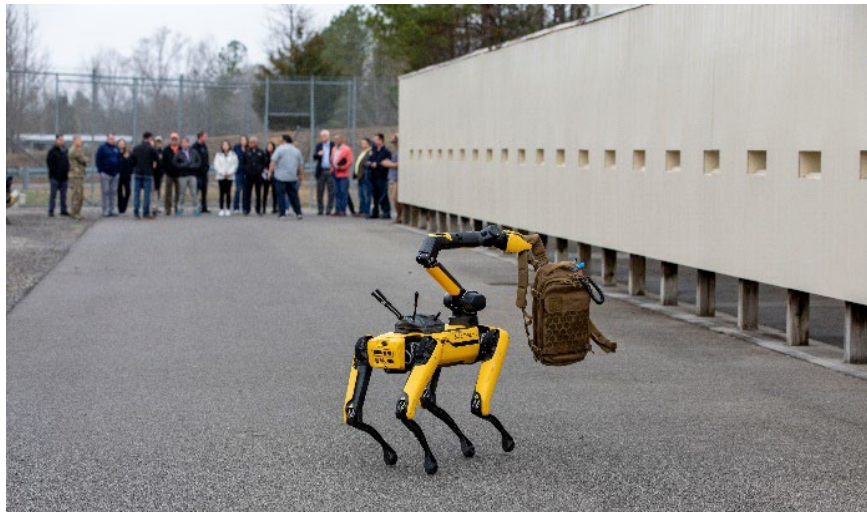
The Y-12 National Security Complex's Spot retrieves a suspicious package while personnel monitor from a safe distance.
