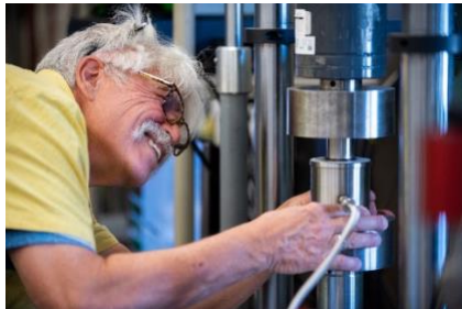
Steve Bauer, a recently retired Sandia Labs geoscientist, is preparing his sensitive mass spectrometer to detect the gases released by crushing a piece of granite. (Photo by Craig Fritz)
