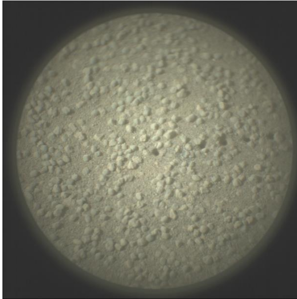
Mars Perseverance Sol 546 - SuperCam Camera: This SuperCam Remote Micro-Imager (RMI) image shows the Red Mountain target, which was analyzed on September 2 (sol 546) as part of a campaign to detect frost at Jezero Crater. The small 'pits' seen in the center of the image were created by LIBS laser shots. (Image Courtesy: NASA/JPL-Caltech/LANL/CNES/IRAP)
