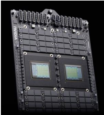
Figure 1. The Vera Vera CPU "Super-Chip" of Ranger (image credit: NVIDIA)
