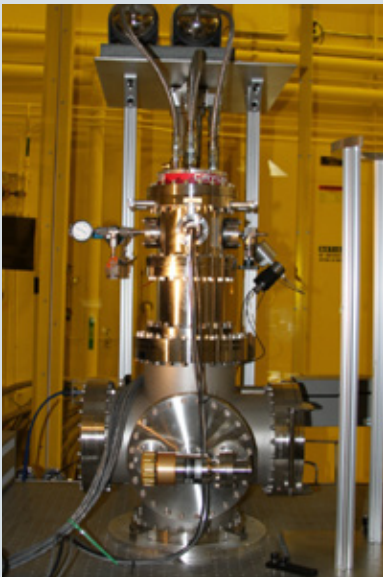
Cryostat used to measure depressed freezing temperature of hydrogen isotopes in ultralow-density foams used in inertial fusion targets. Specifically, we examined the depressed freezing of deuterium–tritium in foams to qualify a liquid and deuterium–tritium layer with low vapor pressure.
