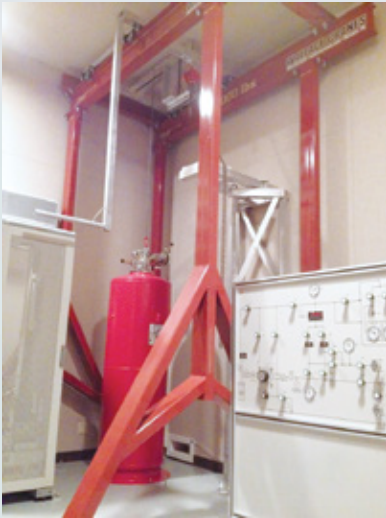
Insert and dilution refrigerator to study fundamental noise mechanisms in superconducting devices in high electric fields and at ultralow temperatures.
