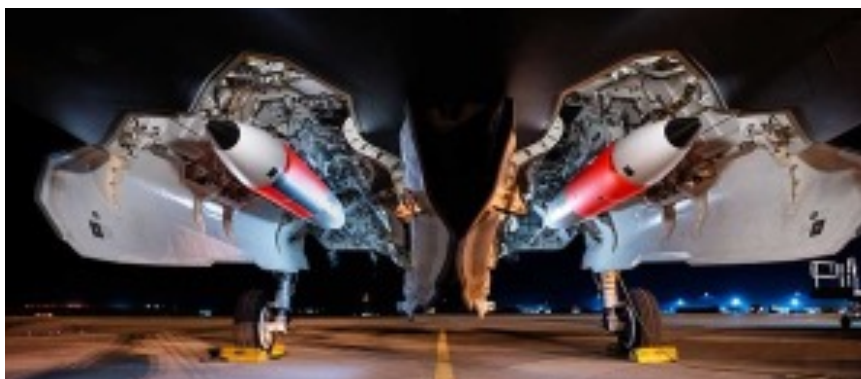
Two B61-12 joint test assemblies loaded on an F-35 aircraft for a flight test on Aug.19, 2025. (Photo by Craig Fritz)
