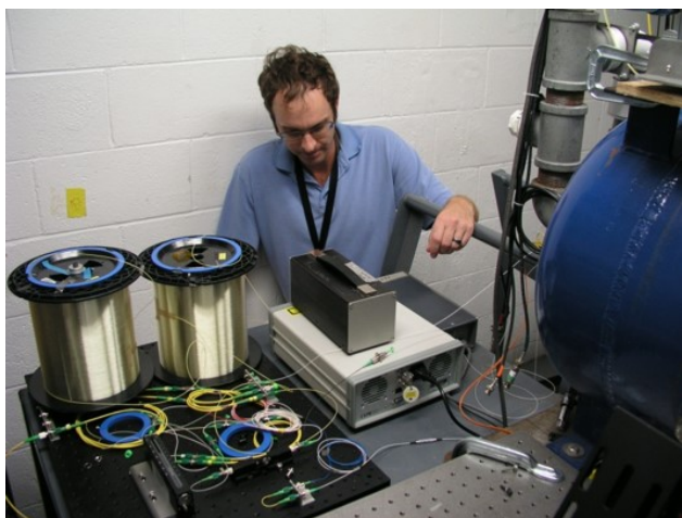
Photograph of the first Broadband Laser Ranging system ever fielded on a dynamic experiment, with Principal investigator Brandon La Lone. (Image courtesy of NNSS.)
