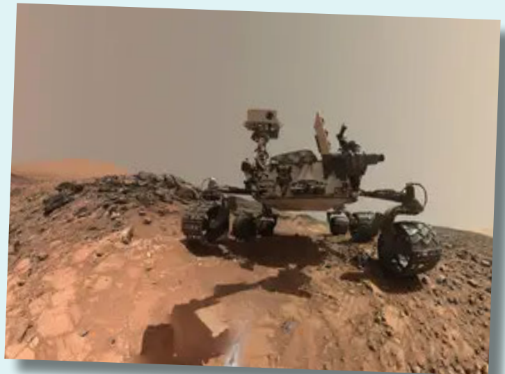
Mars Curiosity with CHEMCam. Photo credit: Reuters/NASA/JPL
