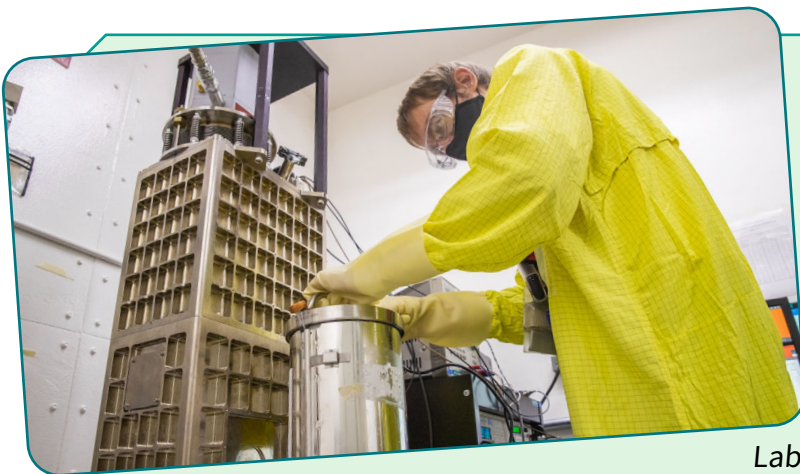
Above: Prototype instrument pictured used to develop a next-generation rapid and nondestructive nuclear material accounting measurement technique to improve the efficiency of operations at the Nation's only Plutonium Facility. Photo credit: LANL
