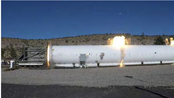
A test explosion in the LANL Blast Tube Facility showing the slight products venting at the tube sections. The aim of this project is to distribute the explosion over the whole length of the tube rather than as a single monolithic explosive charge as used in this particular test.
