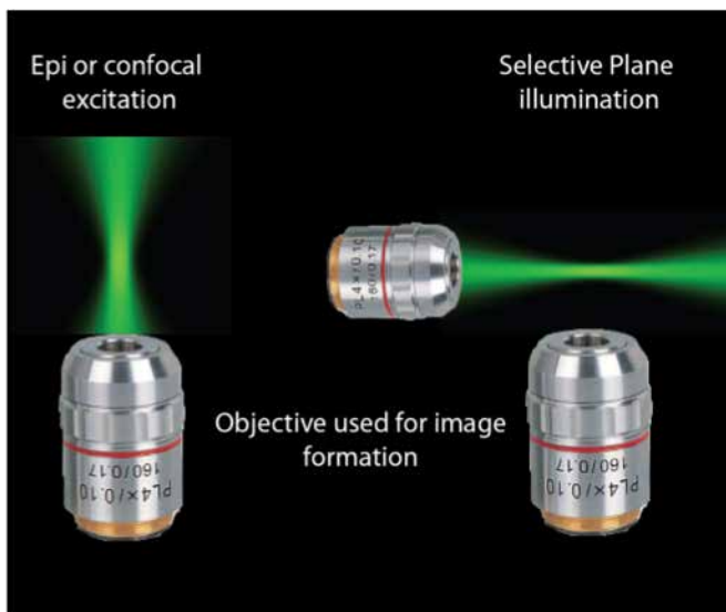
Figure 2. A cartoon comparing epi excitation and selective plane illumination. Selective plane illumination has less
