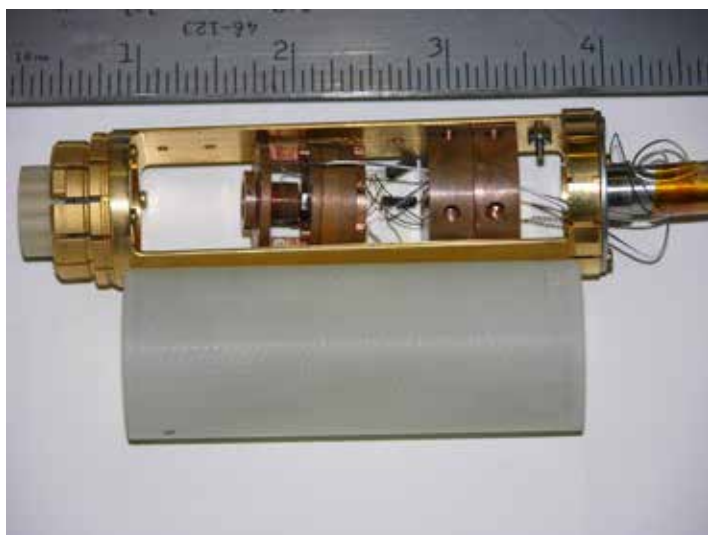
Figure 5. The assembled low temperature dilatometer to measure thermal expansion. The design was based off of the model proposed by Schmeideshoff [7]. The G10 sleeve allows for an encapsulated setup for measuring actinide materials safely in the physical property measurement system (PPMS).
