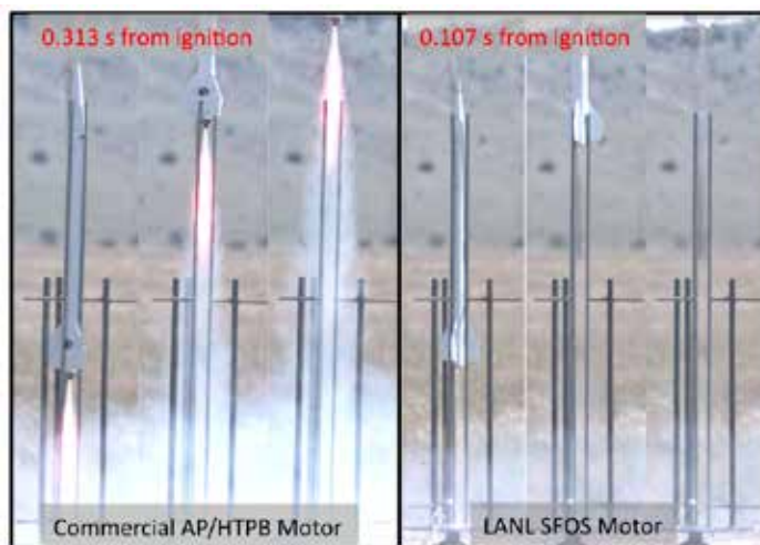
Figure 4. Frame sequence of the commercial (AP/HTPB) baseline motor lifting off the pad vs the LANL SFOS motor.
