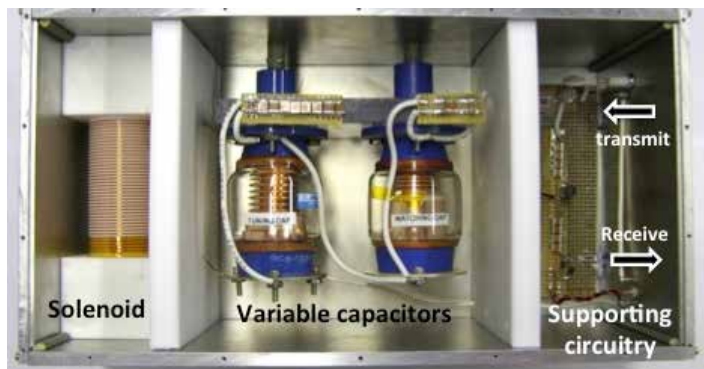
Figure 1. A photograph of our NQR system developed for this LDRD project.
