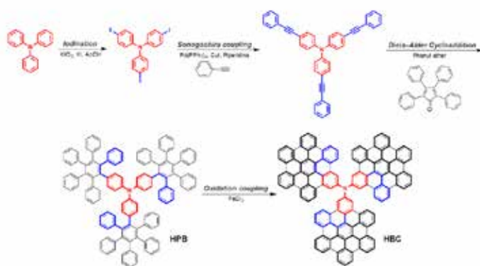
Figure 1. Synthetic scheme of triarylamine (TAA) consists of three nanographene flakes.
