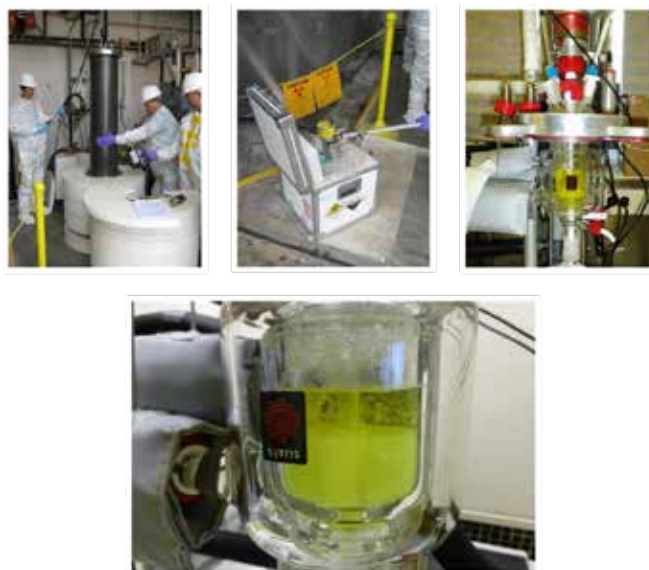
Figure 2. Examples of experimental apparatus used during the course of this project. Top left – the Target 4 capability at LANSCE for LEU solution sample irradiations. Top center – the sample containment for the irradiated LEU solutions, as shown being placed into a Viking shipping container for return to the radiochemistry laboratories for separation chemistry. Top right - the Syrris Atlas Potassium Reactor System used to carefully control the LEU uranium crystallization process. Bottom – a close up of the Syrris Atlas Potassium Reactor System showing the crystallized hydrated uranyl nitrate solid product under a supernatant solution containing significantly less uranyl (and hence uranium) in solution.
