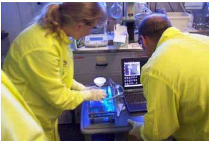
Figure 1. Laura Wolfsberg (C-IIAC) and Jeff Aguiar (MST-8), rehearsing the loading procedure of the Lu-177 TEM sample in to a retractable holder through a shielded plexiglass box. Note the camera providing real time imagery of the sample in the laptop screen.
