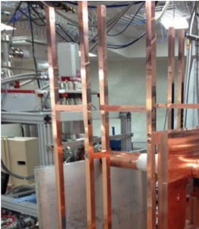
Figure 1. The prototype module just before a detector string was inserted. The large Cu cylinder to the right is the vacuum cryostat that contains the detectors.
