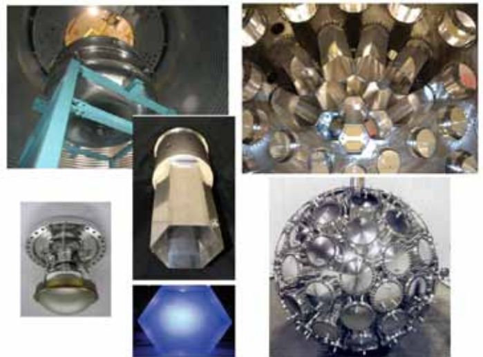
Figure 4. A collage of MiniCLEAN detector components under assembly at SNOLAB: (top left) the Outer Vessel on its stand and inside the water shield tank in the Cube-Hall; (top right) a view of light-guides as they are pre-fit into the Inner Vessel; (bottom left) a PMT assembled in its holder along with the light-guide and acrylic plug with wavelength shifter; (bottom right) the Inner Vessel that serves to hold the cryogenic target and 92 optical cassettes.
