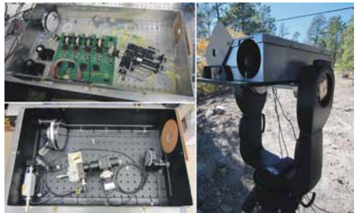
Figure 1. Transmitter (top left and right) and receiver (bottom left) nodes near the completion of the development stage (left) and in the field (right).
