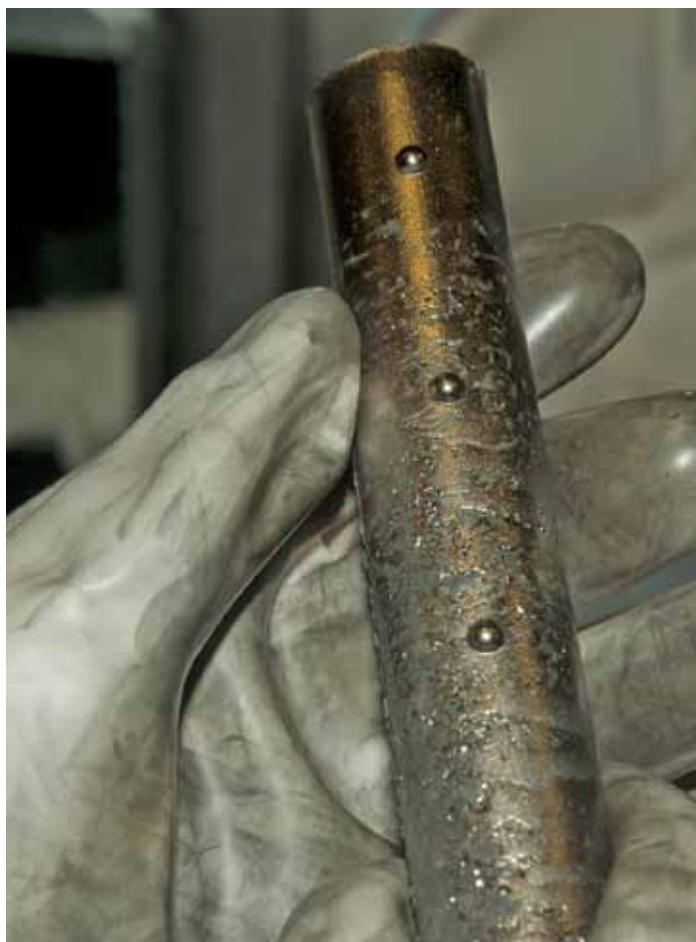
Figure 1. A portion of the Pu-7 atomic % Ga casting produced for this project.
