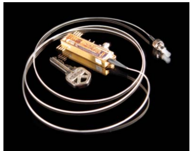
Figure 3. Generation 1 quantum smartcard or QKard. (See text for details.)
