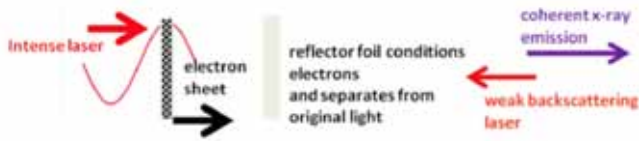
Figure 1. Schematic depiction of laser-based coherent x-ray generation by coherent Thomson backscatter from a relativistic electron mirror. Left: The intense laser incident on a nanofoil target makes an electron sheet moving forward with a relativistic factor \gamma , and traverses the target. That sheet would not support coherent scattering due to finite lateral momentum imparted by the laser on first passage. The laser, upon reflection and traversal through the sheet in the opposite direction, nearly cancels the transverse momentum on the sheet, leaving only longitudinal momentum, making it capable of coherent scattering. Right: A relatively weak backward propagating laser is upshifted to a frequency 4\gamma^2 , i.e., a coherent x-ray pulse.
