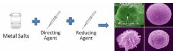
Figure 2. Schematic illustration of the synthesis of metal particles with well-defined morphologies aided by reducing and directing agents. Variations of the molar ratio between reducing and directing agents, and the timing of adding directing agent to the solution can result in metal particles with four distinct morphologies.
