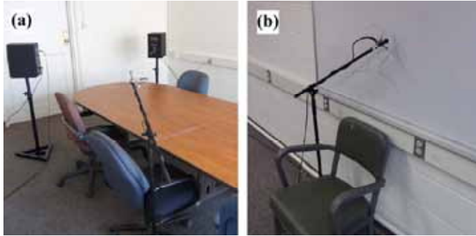
Figure 3. Photographs of the conference room setup used for demonstrations of audible private communications. (a) Photo of two of the loudspeakers used and the microphone placed at a seat location. (b) Photo of a small laser spot shining on a white board above a chair with an outline of a hostage drawn on the board (note that the microphone was placed at the same location in order to record what one would hear at that location).
