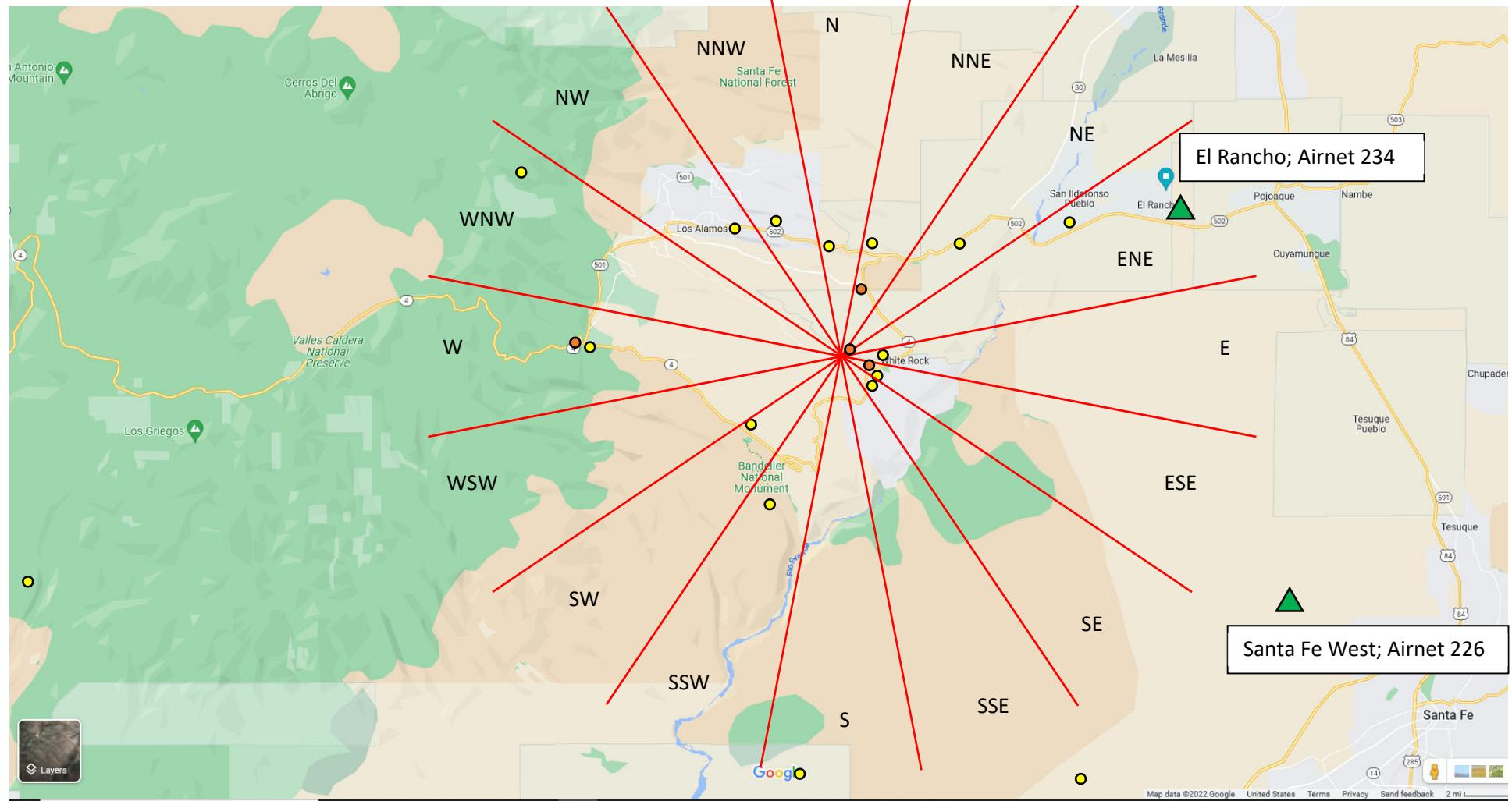
Red: TA-54 Building 1028, FTWC Vent Location; 16-sector grid centered on that location. Vent stack is monitored for tritium releases.
