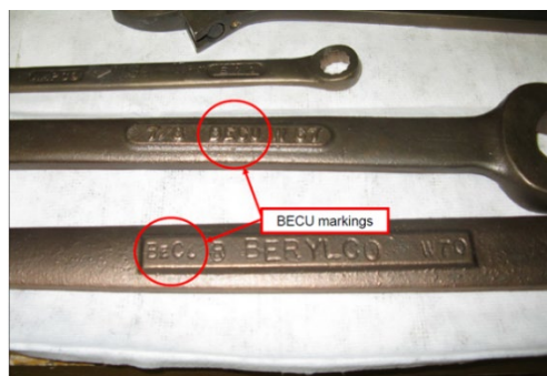
Top left: Elemental beryllium cylinder Bottom left: Beryllium-copper alloy wrenches showing BeCu markings Right: CuBe Fingerstock (1.3% beryllium)
