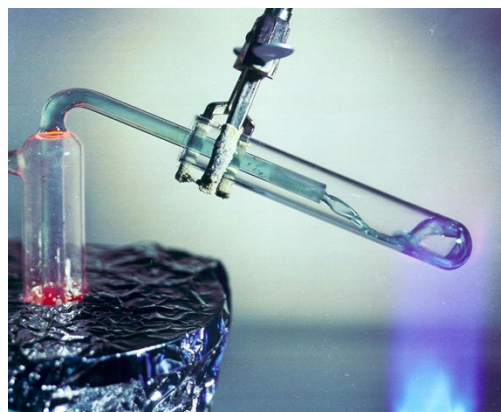
Right - FLiBe is a molten salt made from a mixture of lithium fluoride (LiF) and beryllium fluoride (BeF 2 ). It is both a nuclear reactor coolant and solvent for fissile material (Oak Ridge National Laboratory).
