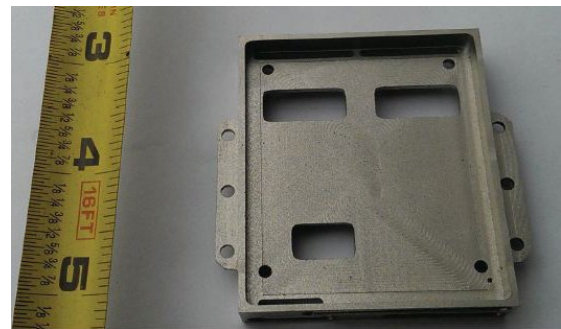
F-35 aircraft component using coated metal powders as a substitute for beryllium materials. (Air Force Research Laboratory)
