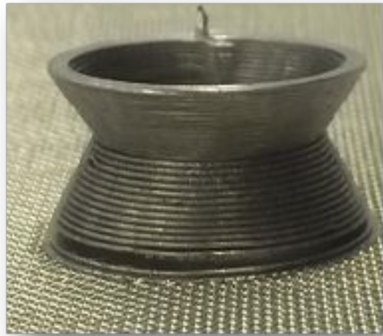
Figure-3: A layered Structure of a 3D component.
