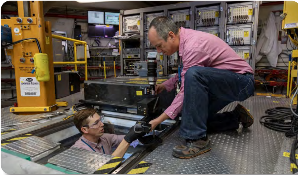
Los Alamos instrument scientists Alex Long (left) and Sven Vogel (right) install the LumaCam event-mode camera onto the High Pressure Preferred Orientation (HIPPO) diffraction flight path at the Lujan Neutron Scattering Center at LANSCE.
