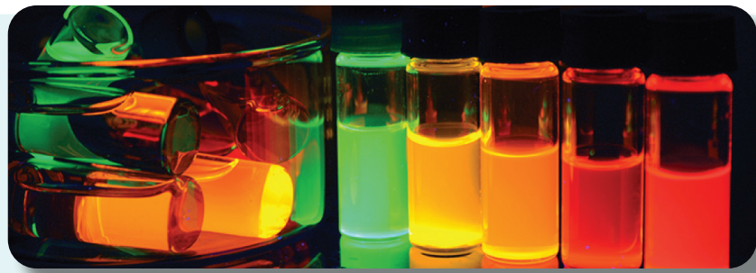
The tiny specs of matter called quantum dots can be tuned to emit light at specific wavelengths. That's just one quality that makes them valuable in a range of technology applications.
