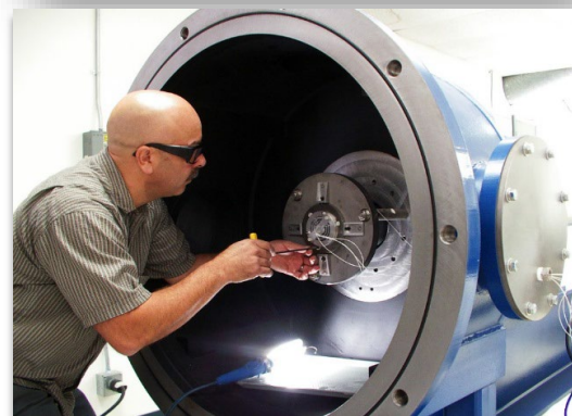
The new propellant launcher, installed in Building 229 at STL, is capable of launching projectiles at 0.5 to 2.5 km/s, which expands the velocity range considerably for shock compression experiments. (Top) Propellant Launcher; (Center) Containment Vessel; (Bottom) Aligning business end of Propellant Launcher in the Containment Vessel.
