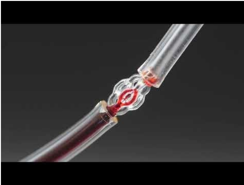
Volumetric additive manufacturing microtubule structure demonstrating perfusibility. (Graphic courtesy of LLNL)
