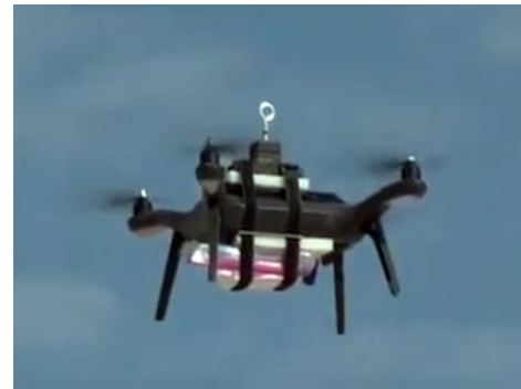
The 3DR UAS with NNSS sensors, flying independently. (Image credit: NNSS)
