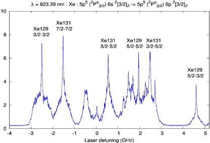
Xenon hyperfine resonance spectra from the rf discharge plasma. The scale of the laser detuning and the peak identifications are preliminary and uncertain.
