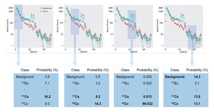
In this same example as above, the <sup>60</sup>Co spectra are now piecewise analyzed by the machine and individual probabilities assigned—the resulting overall analysis is the same, but now the human spectroscopist can see the machine's reasoning.
