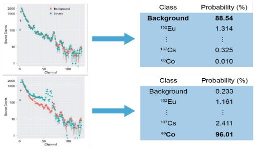
*The two spectra show clearly identifiable sources: one background and one* <sup>60</sup>Co. *The machine classification is correct, but no reason can be assigned by the human analyst.*
