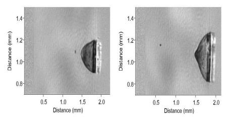
Images from the LIPIT system as part of Staska et al.'s project (STL-025-20) showing a particle being launched by an expanding film bubble. The particle size and velocity are determined from the images.
