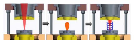
Simplified scheme and time sequence of the proposed technique. The laser beam hits the target mounted on the z pinch generator's cathode plate. A plasma plume is launched across the anode–cathode gap, and then the plume is pinched by a magnetic field on the z-axis.
