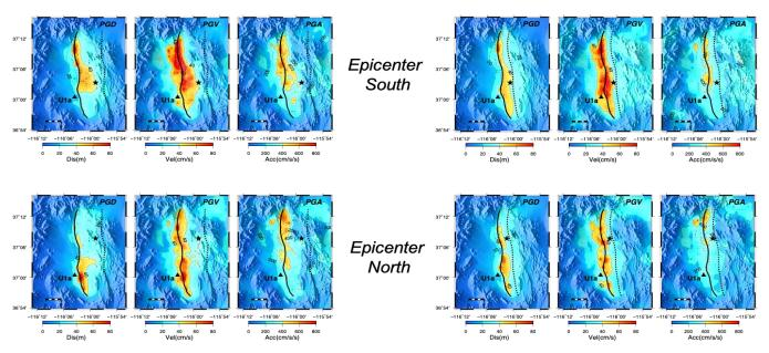
Ground motion simulations of a magnitude 6.5 earthquake on the Yucca fault. The solid black line indicates the surface fault trace; the dashed line is the fault plane at depth. The black star indicates the earthquake epicenter location. Rupture Model 1 assumes a shallow fault geometry, whereas Rupture Model 2 assumes a steep fault plane. PGD is peak ground displacement, PGV is peak ground velocity, and PGA is peak ground acceleration of a single scenario at the surface.
