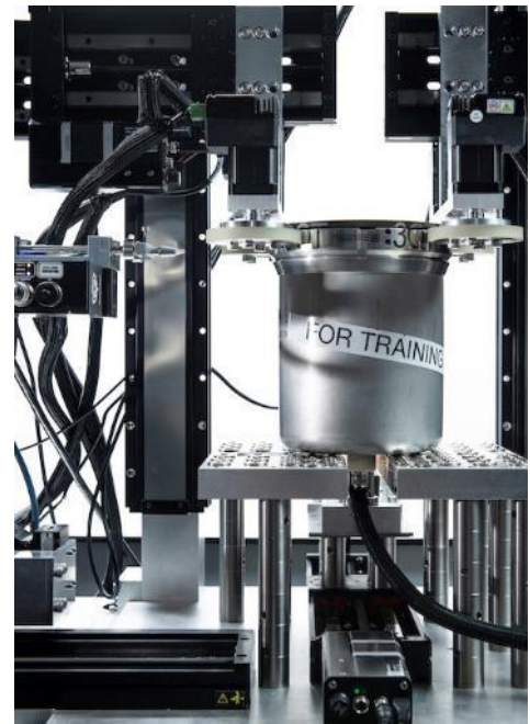
A SAVY container, which holds nuclear materials, is non-destructively tested with Ultrasonic and Laser Interferometer on the left, while Eddy Current Detectors traverse the bottom surface of the container.
