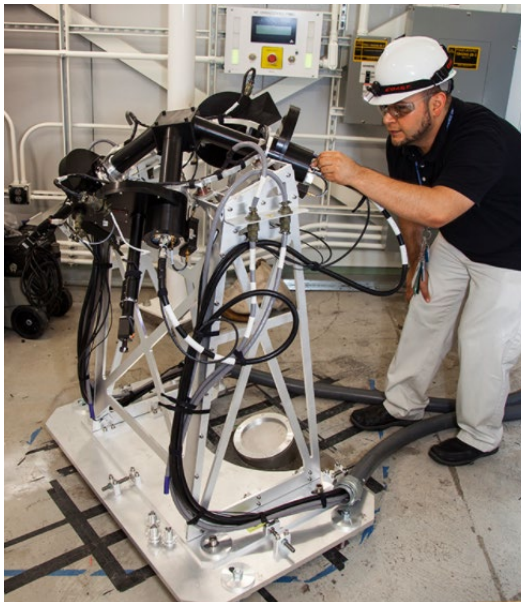
Diagnostics engineer Francisco Barbosa checks a neutron time-of-flight detector at NIF. (Image courtesy of LLNL/James Pryatel.)
