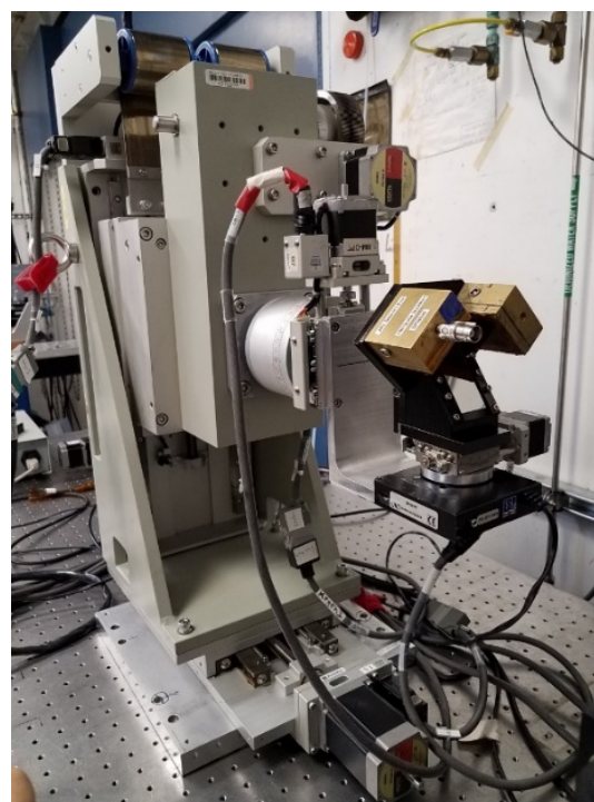
The XRPBS with silicon diode detectors installed on a goniometer for synchrotron measurements.
