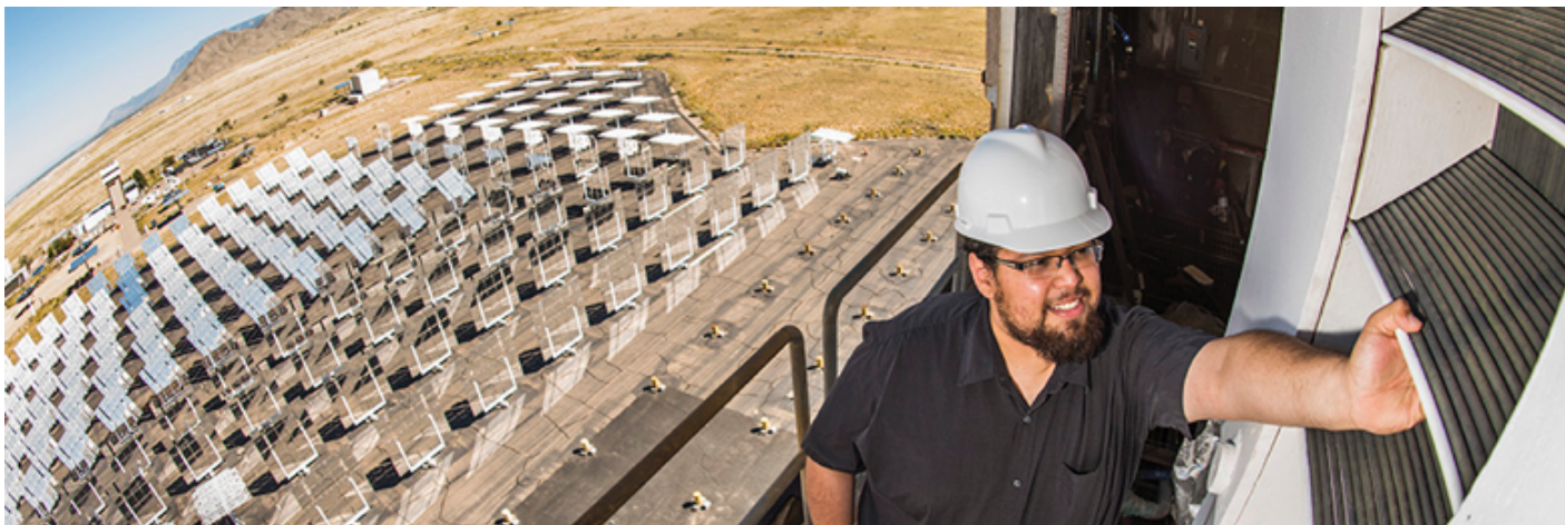
NEW SOLAR RECEIVERS. Year-round Sandia intern Jesus Ortega inspects one of the new bladed receivers at the National Solar Thermal Testing Facility. (Photo by Randy Montoya)
