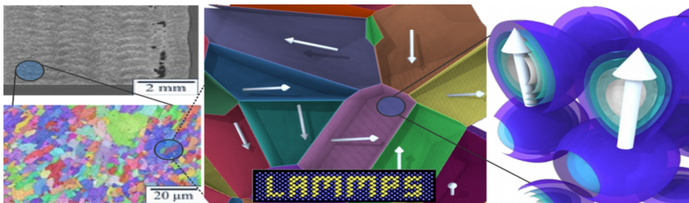
Schematic overview of the multiscale framework bridging between ab-initio and device-level atomistic magnetic simulations. On the left, zoom-in on experimental observations. The middle and right images represent the numerical approach embedded in LAMMPS.
