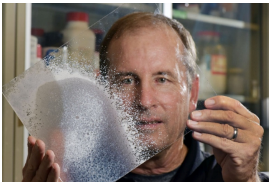
Sandia engineer Mark Tucker holds a sample of decontamination foam modified to stick to the walls and ceilings of subway tunnels. Mark has spent much of the past twenty years thinking about ways to clean up chemical or biological warfare agents. (Photo by Randy Montoya)
