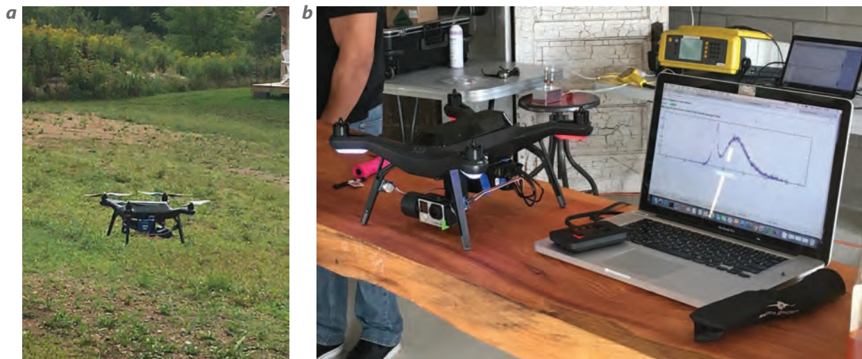
Figure 28. (a) The 3DR Solo carrying the spectrometer in flight and (b) the 3DR Solo with an Ocean Optics Flame-S spectrometer mounted on the expansion bay directly behind the GoPro camera. Mounted behind the spectrometer are the lidar and the Teensy 3.2. The two VOC sensors are mounted on the front legs. The yellow device in the background of the photograph is the GC-MS we used to analyze the smoke samples.
