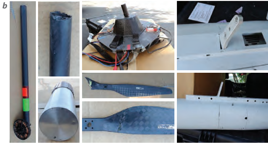
Figure 20. The Virginia Tech hexacopter crashed during a radiation survey flight at the RRTR in Idaho on July 26, 2018. (a) The flight path up until the crash. (b) Although the aircraft was a total loss, both detectors survived.
