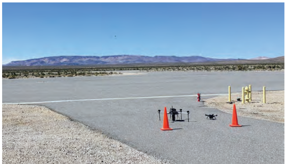
Figure 7. The 3DR Solo carrying the 2x2 NaI detector is hovering over a ^{152}\text{Eu} source at the edge of the runway at the Desert Rock Airstrip. In the left foreground is the ORNL Strelka heavy-lift copter; another 3DR Solo sits to its right.
