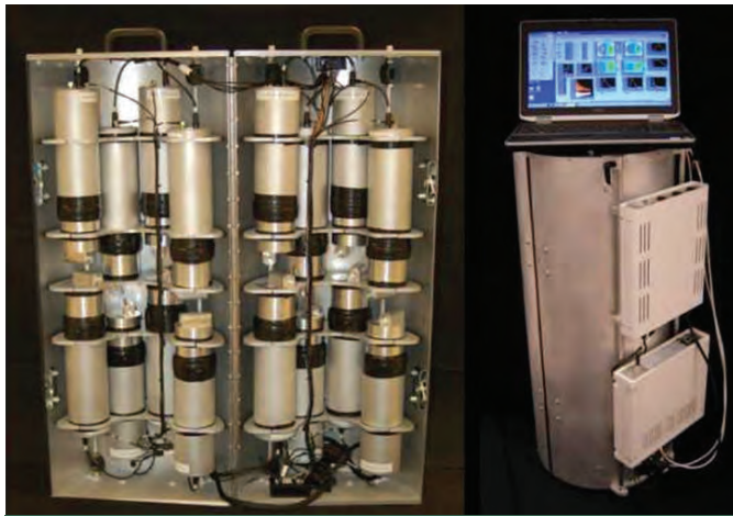
Figure 14. The SNL MINER detector array system will be used in our FY 2019 tests to detect HEU
