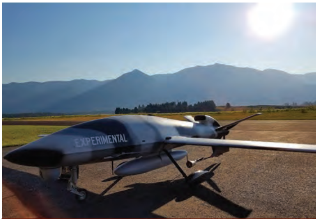
Figure 21. The chemical sensor pod was mounted to the belly of the Sandstorm, and the air sampling tube and VOC sensor chip were mounted below the left wing
