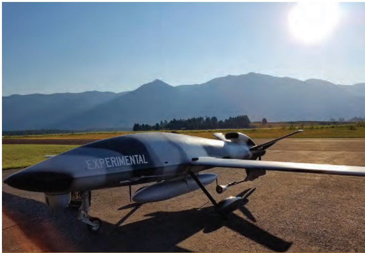
Figure 2. The detector pod for chemical or radiation detection is attached to the belly of the Sandstorm.
