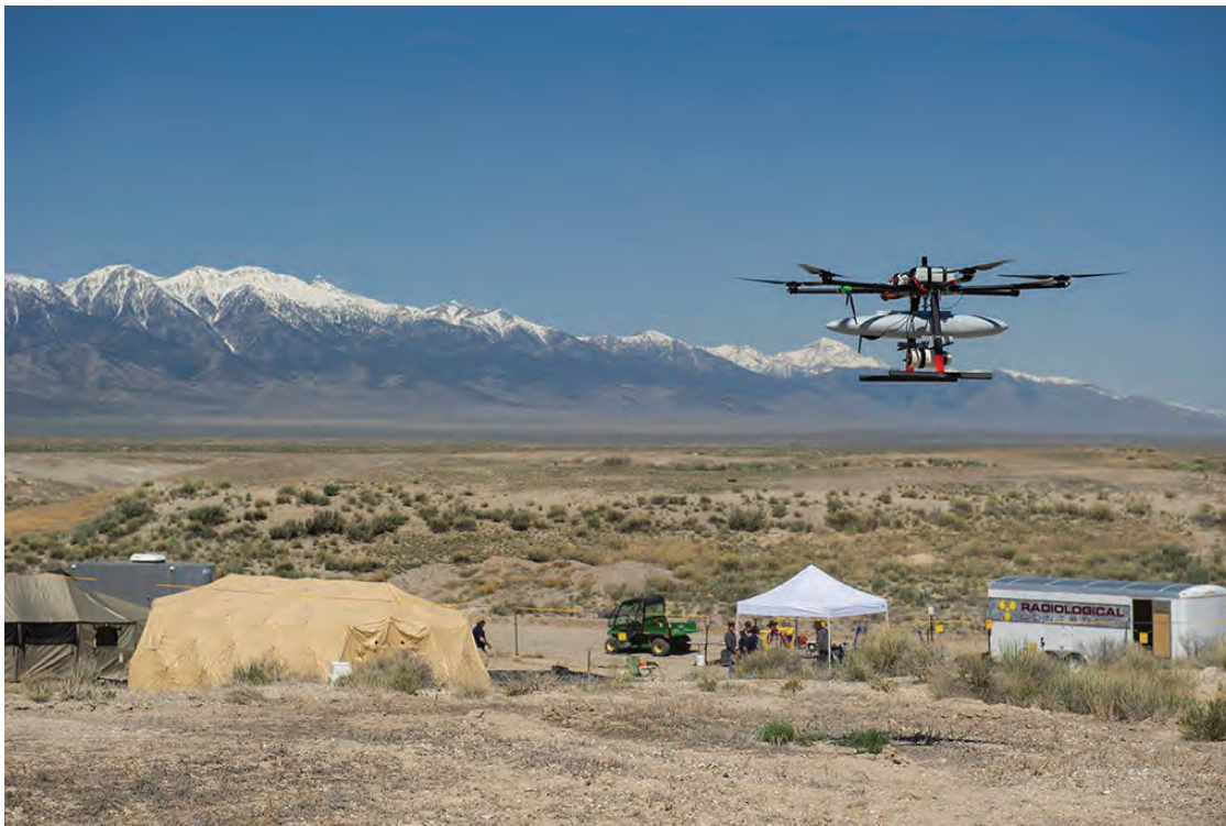
Figure 10. The Virginia Tech hexacopter carries the Apollo detector and the Raspberry Pi in the pod mounted beneath it, and the 2x2 NaI detector is mounted beneath the pod. This photo was taken in April 2018 at an exercise in Idaho.
