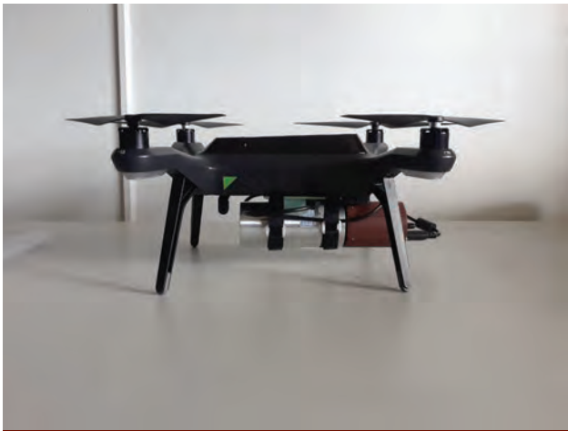
Figure 16. The modified, “stubby” 2×2 NaI(Tl) detector is strapped to the bottom of a 3DR Solo. The detector is controlled by the Solo’s onboard i.MX6 computer.
