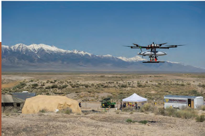
The Virginia Tech hexacopter carries the Apollo detector and the Raspberry Pi in the pod mounted beneath it, and the 2x2 NaI detector is mounted beneath the pod. This photo was taken in April 2018 at an exercise in Idaho.
