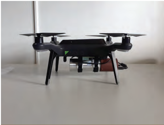
Figure 6. The 3DR Solo quadcopter with a 2x2 NaI gamma detector strapped to it has been flown in tests in Nevada and Montana. Similar 3DR Solos with a chemical detector and an optical spectrometer have been flown in Wisconsin.
