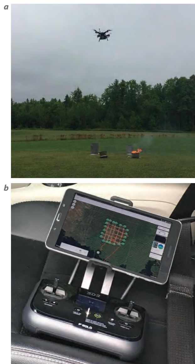
Figure 25. (a) The 3DR Solo quadcopter flying over garbage cans filled with kerosene-soaked burning rags. (b) The 3DR controller with the tablet computer showing the flight plan uploaded to the 3DR Solo.
