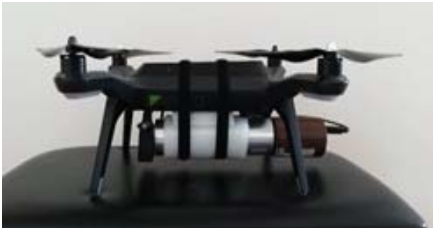
Figure 7. 2x2 NaI:Tl gamma detector on the 3DR Solo Quadcopter
