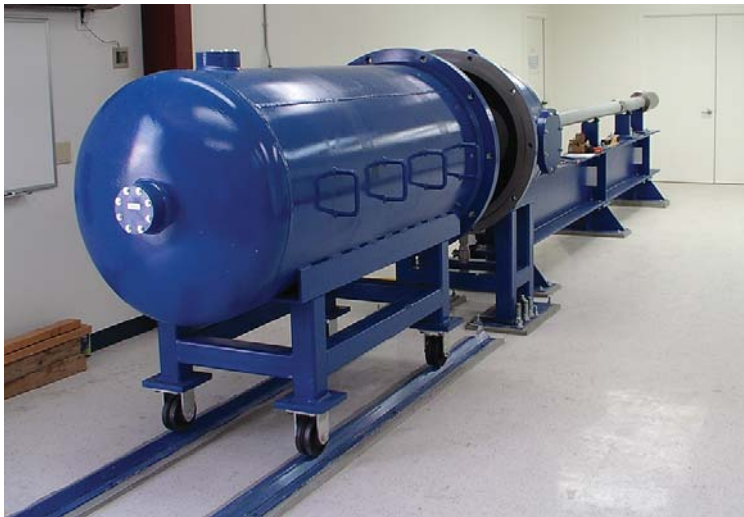
Figure 7. The new propellant launcher, installed in Building 229 at STL, is capable of launching projectiles at 0.5 to 2.5 km/s, which expands the velocity range considerably for shock compression experiments
