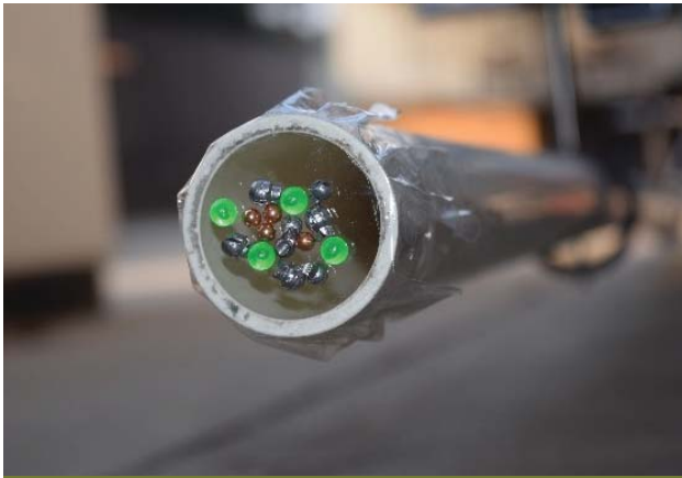
Figure 8. PVC vacuum launcher configured with lead, steel, and plastic targets
