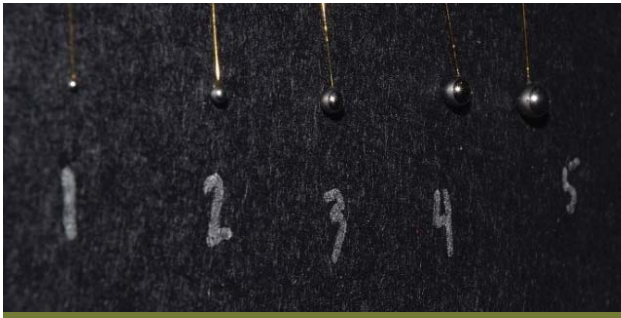
Figure 2. Static test spheres (suspended from thin optical fibers) sized from 1 to 5 mm
