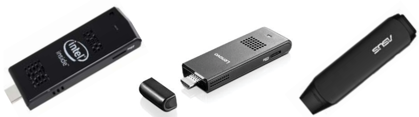
Figure 10. Example stick computers; typical size is 4" × 1.5" × 0.5" and weight of 1.9 oz
