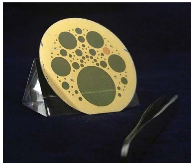
Figure 2. InGaN photocathode devices on 2" sapphire wafer with a range of sizes (20, 10, 4, 2, 1, and 0.4 mm) for testing purposes and eventual detector assembly with a multiplier stack
