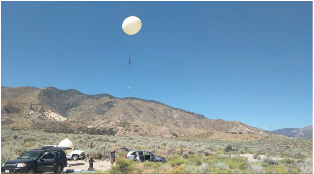
Figure 8. A Canary was launched with a weather balloon to 103,000 feet; data were used for sensor calibration and performance assessment
