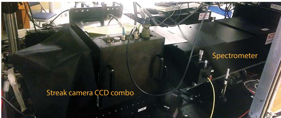
Figure 1. Acton SpectraPro SP-2750 spectrometers coupled to an NNSS-built optical streak camera (L-CA-24)
