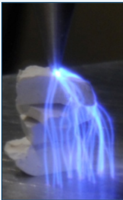
Open shutter photograph of surface flashover near the high dielectric material used in lightning arrester connectors. The event was triggered with a fine wire near the top of the dielectric stack. Photo credit: Zachariah Wallace.
