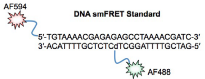
Figure 4. A cartoon depiction of the DNA test sample used to measure smFRET while tracking. The donor (Alexa 488 or AF488) and acceptor (Alexa 594 or AF594) are separated by 12 DNA bases, close enough for efficient Forster energy transfer.
