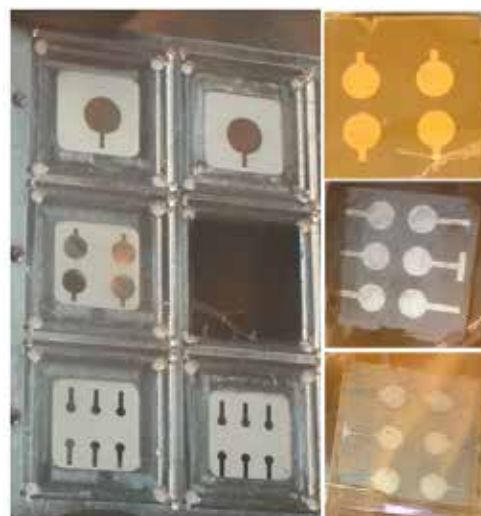
Figure 4. At right, the custom masks for thermally evaporating the metallic top contact of sandwich-type radiation detection devices. Three different device areas can be used (2, 5 and 10 mm diameters); the rectangular tab allows electrical contact to be made using a probe without “shadowing” the active device area. At right, actual devices: simple ITO/NQD/Au sandwich device (top); ITO/NQD/Ag device (middle); and ITO/CuSCN/NQD/ZnO/Al device (bottom).
