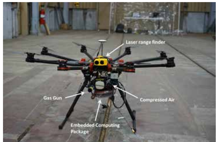
Figure 1. Remote sensor placement device installed on S100 octorotor for testing
