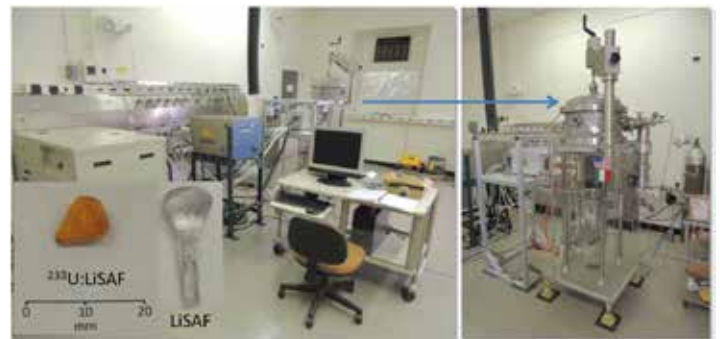
Figure 4. New crystal growth lab at LANL developed under this project. The system is suited for both micro-pulling-down and Bridgman growth of fluoride crystals. The inset shows undoped LiSAF (right) and U-233 doped LiSAF (left) samples grown at LANL using the Bridgman method.
