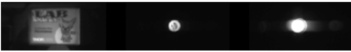
Figure 3. Sample images acquired with the optical system showing typical imaging performance of an extended object (left), a standard spiral-type compact fluorescent bulb with an unsaturated sensor (center) and strongly saturated sensor (left). Images of extended objects reveals small issues with focus across the object, but does not exhibit the mis-alignment of otherwise in-focus images typical of the old-style MMAs. Saturation images show two kinds of artifacts due to critical design parameters of the new-style MEMS array and their relative power to the core image. The near field ghosts are more than 10x times less intense than the core image and will impact the diffraction-limited performance of the sensor.
