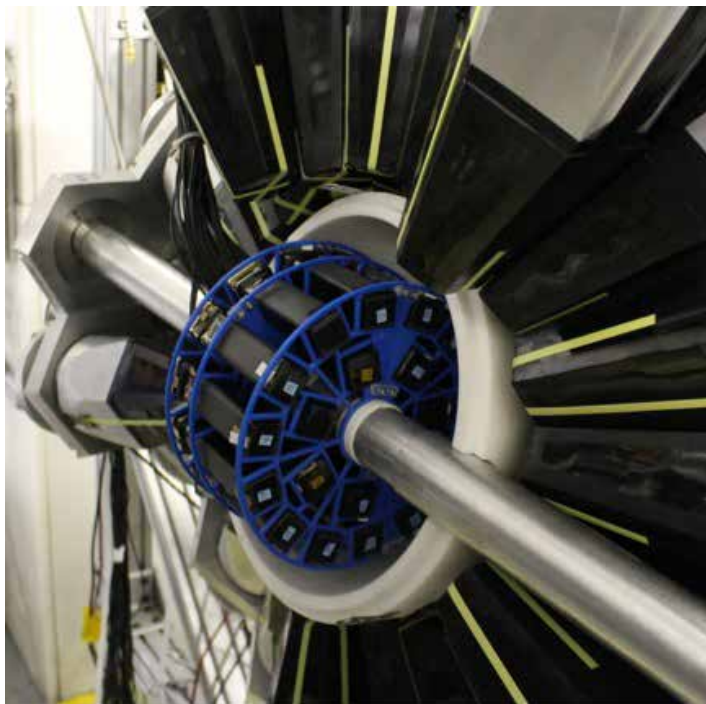
Figure 2. NEUANCE - Neutron detector array consists of 21 stilbene crystals arranged in the cylindrical geometry around the beam pipe. The inner and outer rings of NEUANCE include 7 and 14 detectors, respectively.
