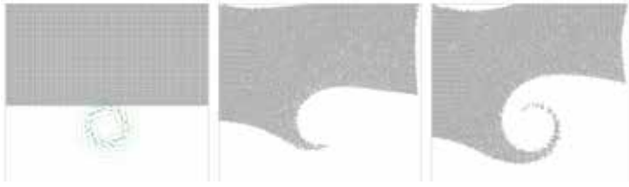
Figure 2. Initial distribution of elements in an idealized test case with a vortex wind field (green). Simulation after 2 days. Simulation after 4 days.
