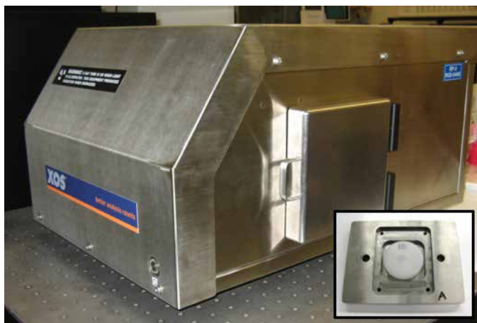
Figure 1. hiRX benchtop prototype instrument and sample microcell in mounting apparatus (inset)
