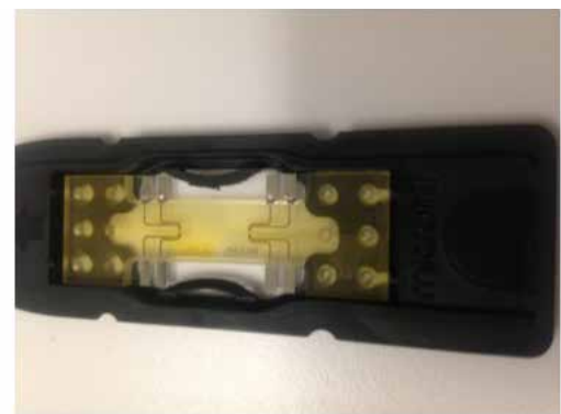
Figure 2. The microchannel device with impedance electrodes integrated and fabricated by Micronit using our design.
