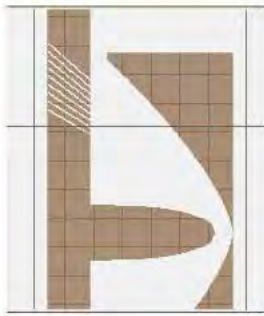
Figure 4. SIMION model showing a shaped pinhole plate and cone-like structure at the filter plate center. The pinhole is located above the center of the cone, and only a limited number of filter plate channels are shown.
