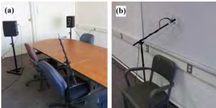
Figure 1. Photographs of the conference room setup used for demonstrations of audible private communications. (a) Photo of two of the loudspeakers used and the microphone placed at a seat location. (b) Photo of a small laser spot shining on a white board above a chair with an outline of a hostage drawn on the board (note that the microphone was placed at the same location in order to record what one would hear at that location).
