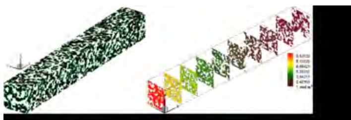
Figure 4. Reconstructed 3D nanoscale structure of a cathode CL (left). Oxygen concentration in the NPMC CL obtained from the LBM simulations (right).
