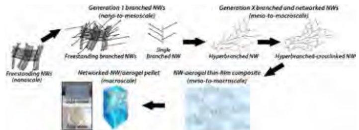
Figure 1. Schematic showing increasing complexity in nanowire structures and integration with aerogel (thermally insulating, structurally supportive) matrix material.
