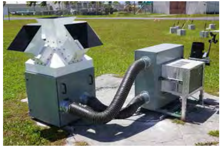
Figure 1. The marine-hardened full-sky optical monitor deployed on Kwajalein Atoll in the Pacific Ocean. This fully autonomous sky monitor was operated for six months without human intervention on Kwajalein. The system collected important Space Situational Awareness measurements and successfully passed it's marine environment testing.
