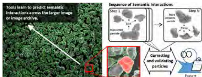
Figure 1. Supervised Semantic tools learn more from experts than standard machine learning tools because they understand semantic interactions like splitting and merging. These interactions are encoded into the Graphical Model and then propagated across the larger data set or data archive.
