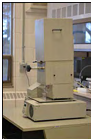
Figure 2. SFT-110 COTS SCCO 2 Extraction System without Separator
