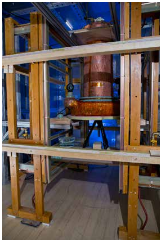
Figure 4. Photograph of the shielded (V1) ULFMRI system.
