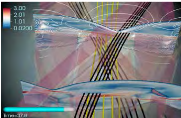
Figure 2. Three dimensional realization of magnetic reconnection illustrating tearing mode mechanism computed using a two-fluid plasma model in a triply-periodic domain. Lines denote magnetic field lines and color map shows charge density.
