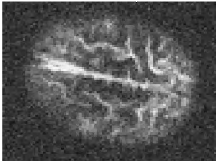
Figure 1. Horizontal (top down) image of the human brain acquired with the Los Alamos National Laboratory ULFMRI system developed with this project. The MRI was acquired at 100 \mu T (about twice the earth’s magnetic field) and 10,000 times less than a conventional MRI.
