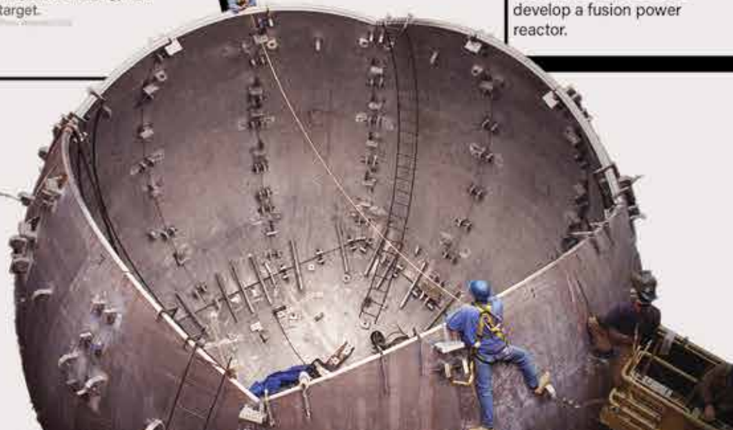
● Inside the Omega laser's target facility at the moment of operation. Omega is a 60-beam system capable of delivering 30 kilojoules of energy to a target.
