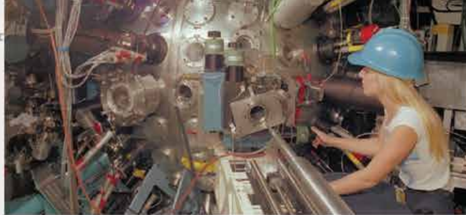
■ Livermore's Shiva laser operated from 1977 to 1981. Its target chamber, which was vacuum sealed and held deuterium-tritium targets as well as experimental diagnostics, is pictured here.
