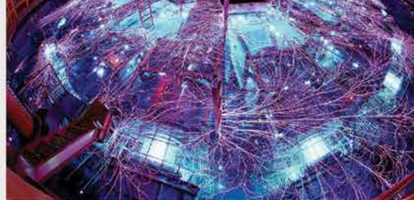
● Sandia's Z machine generates extreme x-ray bursts and pressures to pursue fusion and other research.
