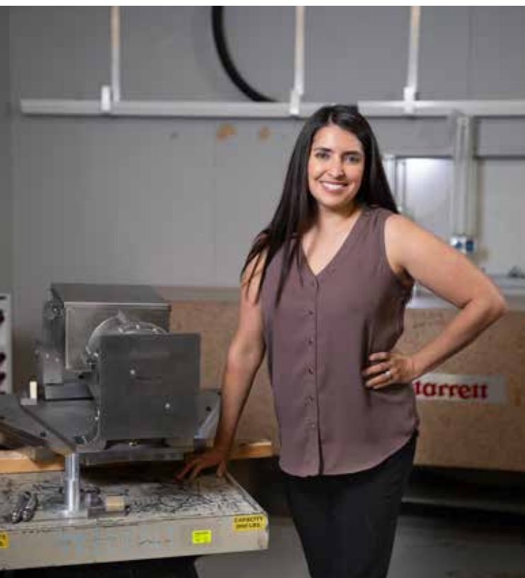
■ Engineer Tana Morrow stands beside nuclear reaction history diagnostic device that provides physics data on the evolution of the burning fusion fuel. Los Alamos researchers developed the device, the Proton Trajectory Assay - Recoil Telescope (PAJARITO), to study thermonuclear burn experiments on the Z machine.
