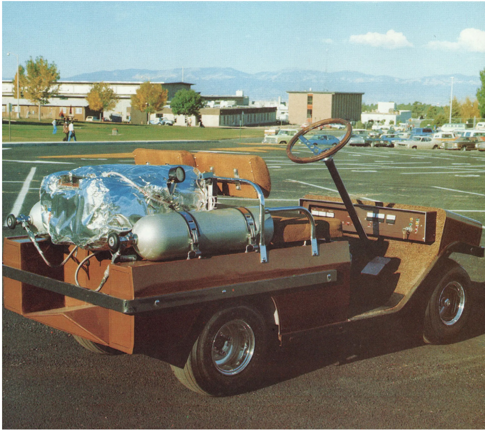
A hydrogen fuel cell golf cart made at Los Alamos Scientific Laboratory in the 1970s.
