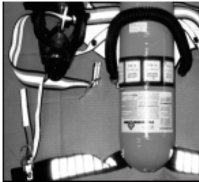
SCBA: full-face, positive-pressure, pressure demand 30 minute unit
