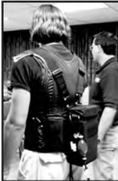
Photo 2: Bottle carrier (r), pump priming bulb (m), and battery pack (l)
