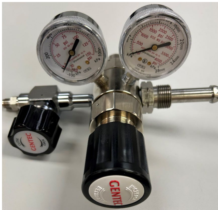
Figure 8: This picture shows a regulator used for compressed air.
