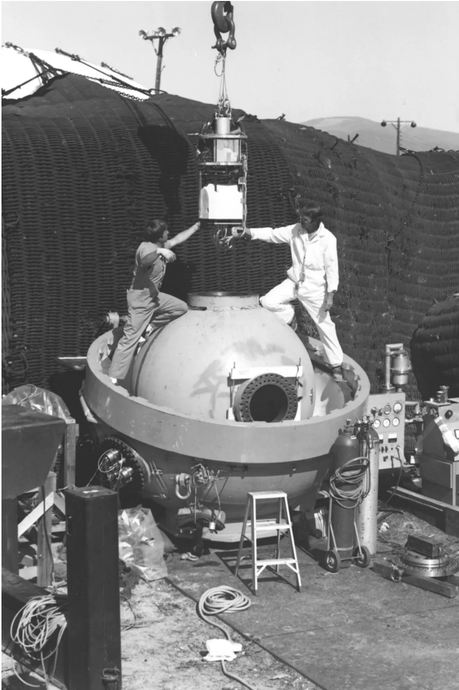
Historical photo of confinement vessel at the Lab's PHERMEX (Pulsed High-Energy Radiographic Machine Emitting X-rays). PHERMEX was used for 40 years to visualize explosions using flash radiography.
