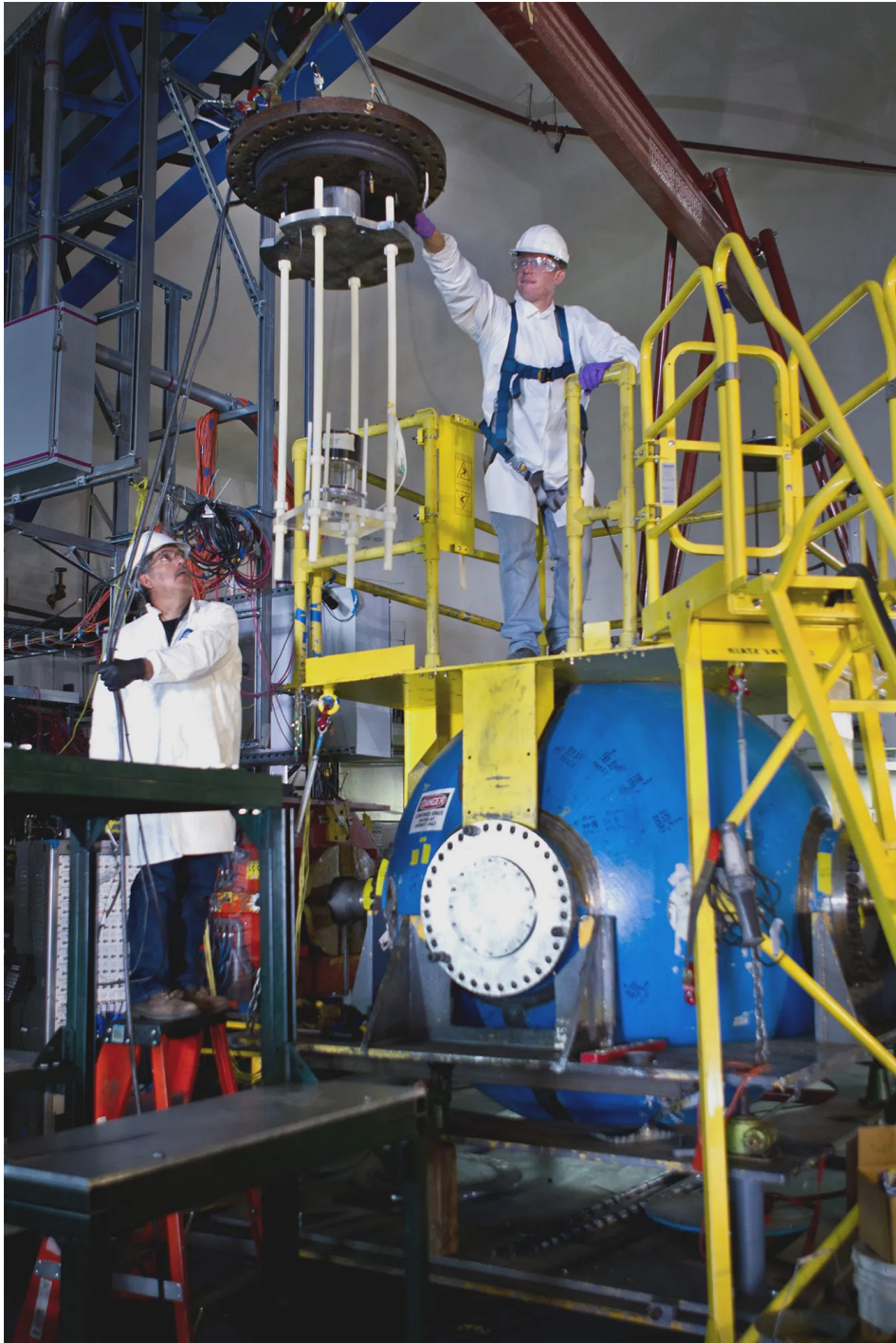
Lowering an experiment into the containment vessel at the pRAD facility at the Los Alamos Neutron Science Center (LANSCE). Los Alamos scientists invented proton radiography to take advantage of the unique properties of high-energy protons to capture multiple images of a detonation.
