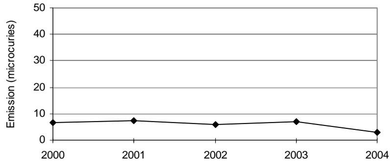
**Figure 4-16.** Uranium emissions from sampled LANL stacks.
