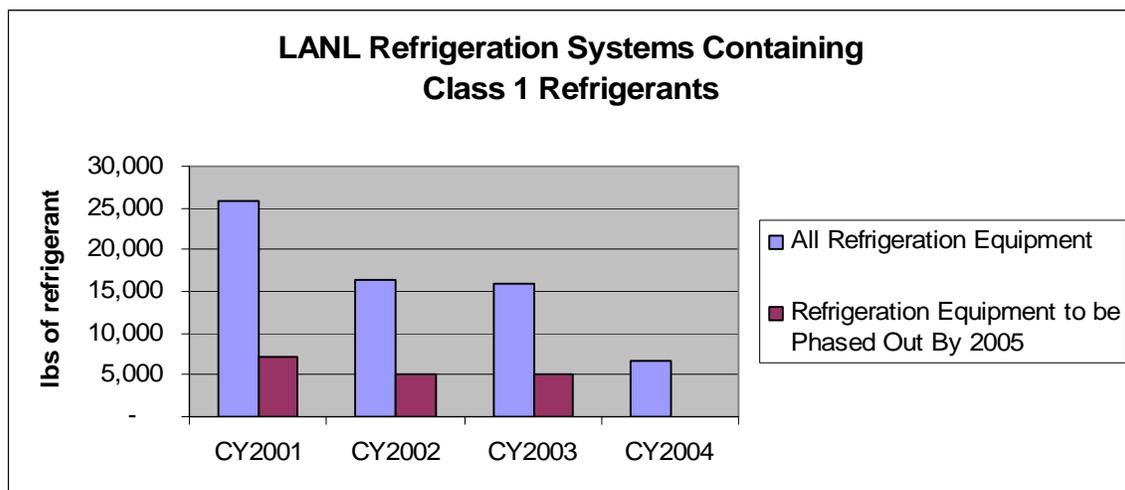
Figure 2-2. LANL refrigeration systems containing class 1 refrigerants.
