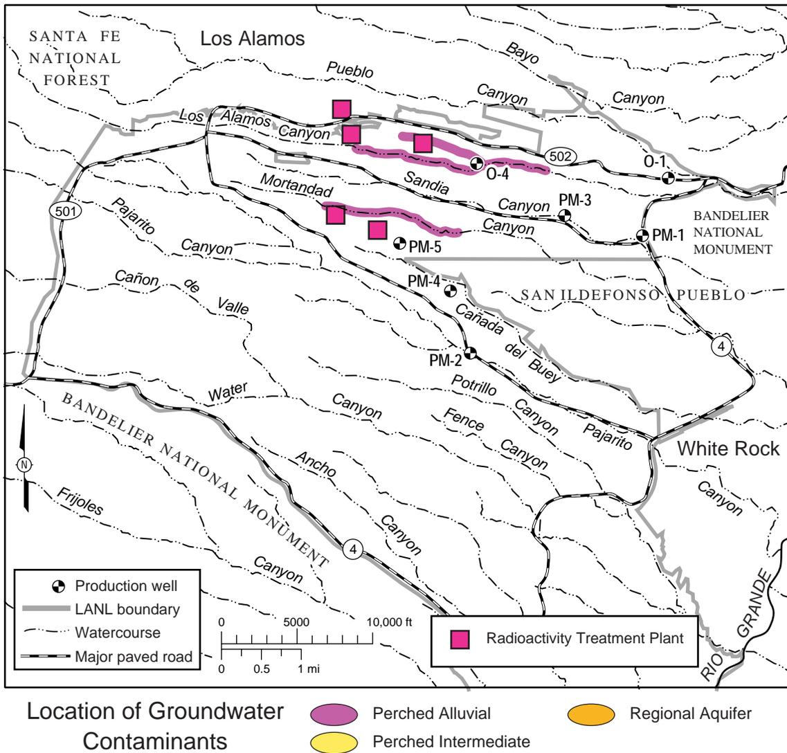
**Figure 5-9.** Location of groundwater contamination by Sr-90 above the 8 pCi/L EPA MCL. The maximum 2004 values in Mortandad and DP/Los Alamos Canyon alluvial groundwater were 7.6 and 4.6 times the MCL, respectively. Different colors indicate the affected groundwater zones. Along canyons, the extent of alluvial groundwater contamination lateral to the canyon is not to scale: contamination is confined to the alluvium within the canyon bottom and is narrow at the map scale.
