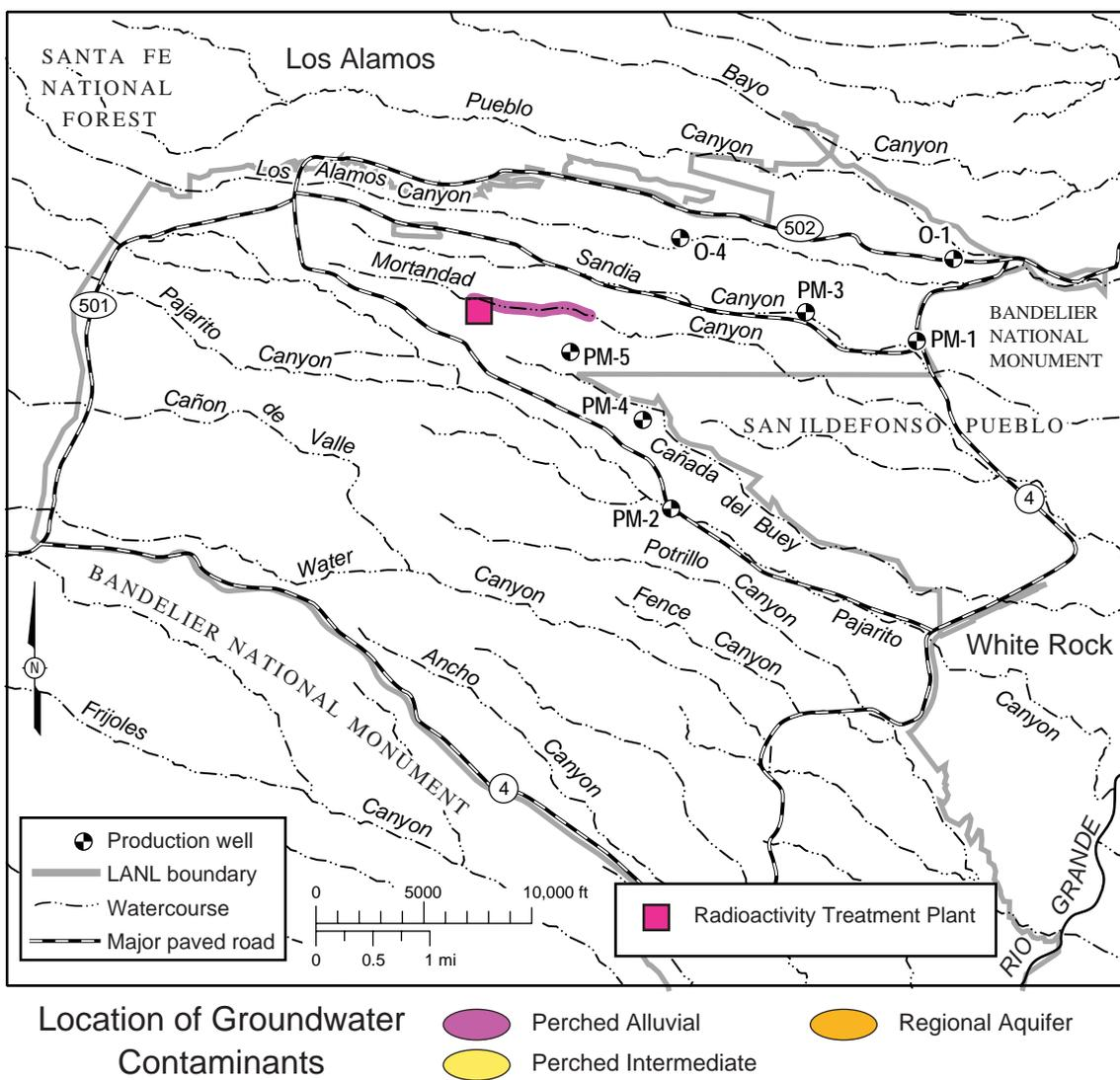
**Figure 5-10.** Location of groundwater contamination by the sum of Sr-90, Pu-238, Pu-239,240, and Am-241 above the 4-mrem DOE DCG for drinking water. The 2004 maximum values in Mortandad Canyon alluvial groundwater for Sr-90, Pu-238, Pu-239,240, and Am-241 were 1.53, 0.35, 0.35, and 0.47 times the 4-mrem limit, respectively. Different colors indicate the affected groundwater zones.
