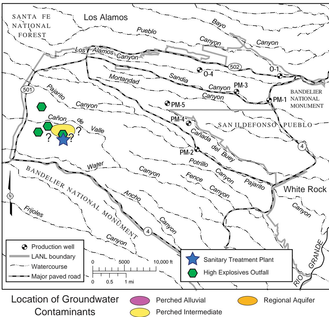
**Figure 5-19.** Location of groundwater contamination by RDX above the EPA Region VI screening level of 6.1 ppb in perched intermediate groundwater. Maximum 2004 values for RDX in intermediate groundwater at well R-25 were seven times the 6.1 ppb EPA Region VI 10-5 excess cancer risk screening level. Different colors indicate the affected groundwater zones.
