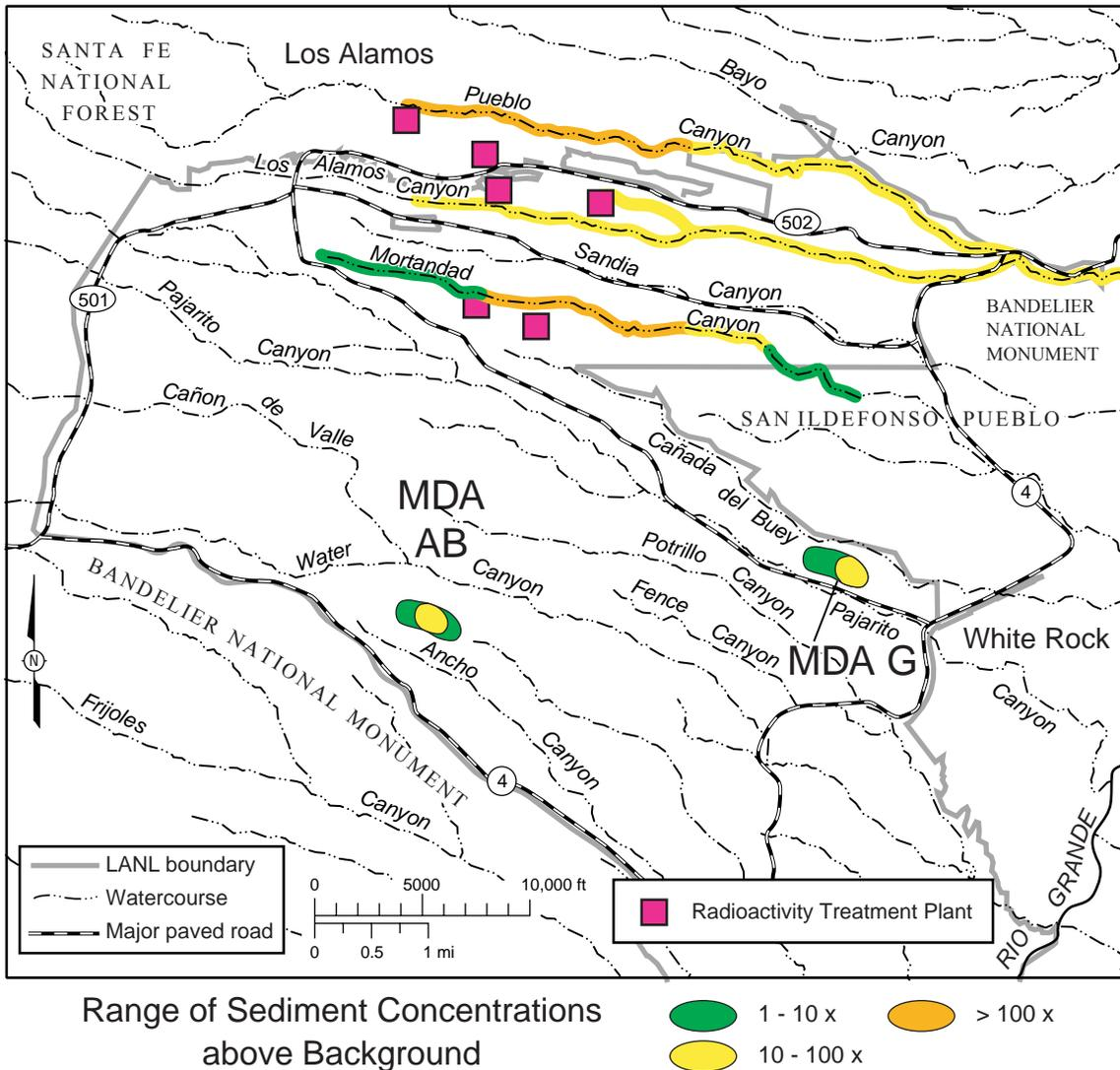
**Figure 6-10.** Location of the active stream channel sediment with Pu-239,240 activity above the fallout levels derived from McLin and Lyons (2002). Different colors indicate the proportion of concentration to the fallout level. Shaded squares show locations of past or current radioactive effluent sources (see Chapter 5 in text). The highest value in 2004 was in Mortandad Canyon, at 758 times background, 22% of the residential SAL, and 16% of the industrial worker SAL.
