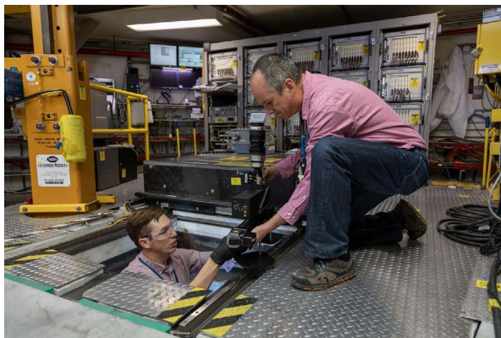
Los Alamos instrument scientists Alex Long (left) and Sven Vogel (right) install the LumaCam event-mode camera onto the High Pressure Preferred Orientation (HIPPO) diffraction flight path at the Lujan Neutron Scattering Center at LANSCE.
