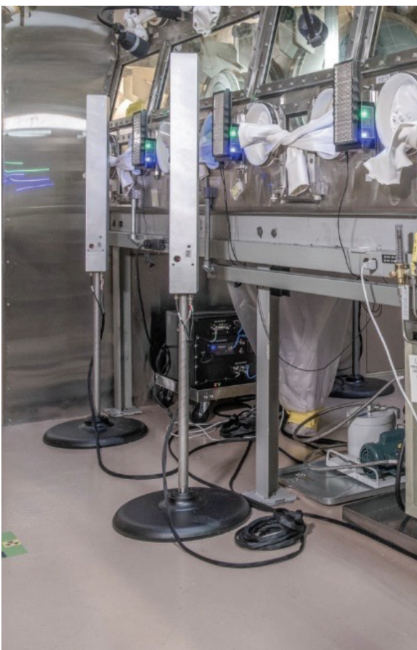
Figure 7. Neutron detectors on flagpole stands, part of the DBCM system deployed at a glovebox in PF-4.
