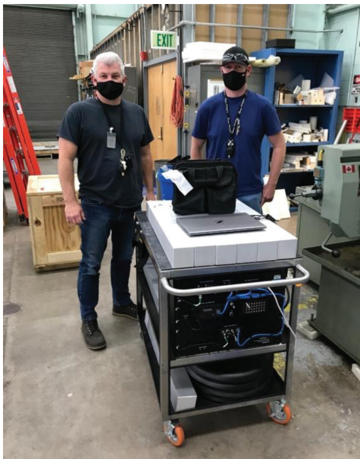
Figure 6. (a) DBCM packed on the cart (six neutron detectors visible as white rectangular boxes on the upper tray); (b) Components of a single neutron detector, which is positioned on a flagpole as part of the DBCM system.
