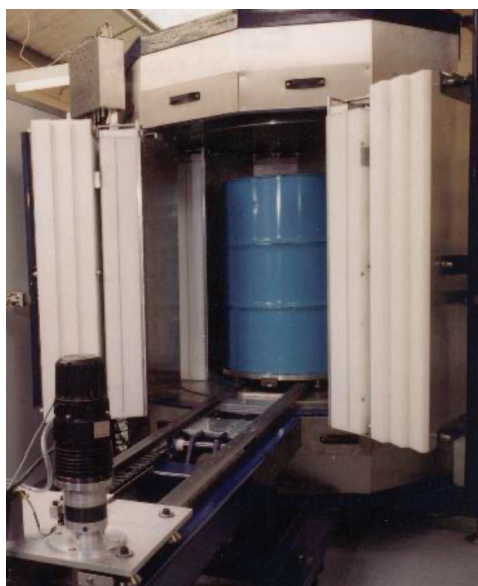
Figure 2. Transuranic waste in PF-4 is currently bagged out into a 55-gallon drum, assayed in the NDA laboratory, and then measured again with a high efficiency neutron counter (an example instrument pictured). Currently, this inefficient process involves moving waste three times. Credit: Antech.
