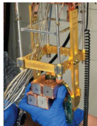
Sideways-facing microsnouts with 400 pixels shown as installed in the cryostat of HERMES.
