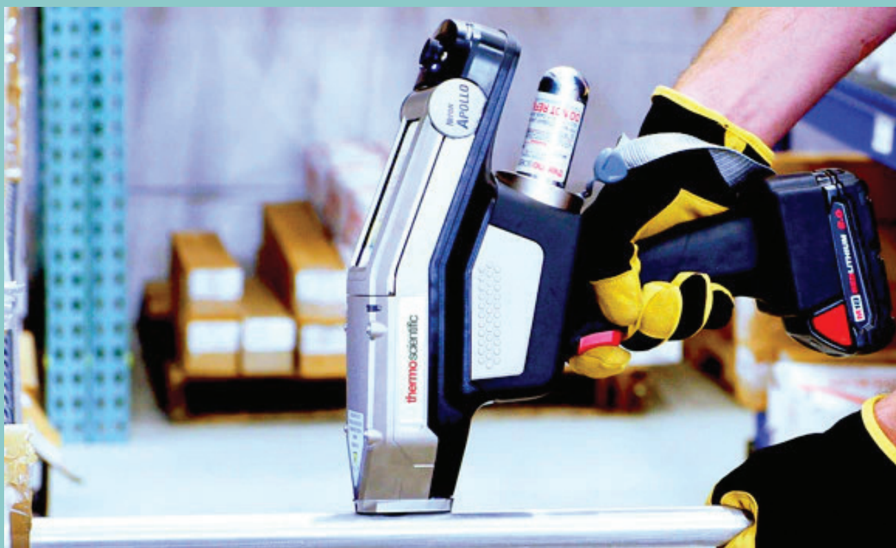
Above: The portable laser-induced breakdown spectrometer (LIBS), used for homeland security, emergency response, and environmental monitoring of hazardous materials, is an example of an NDA safeguards innovation developed at Los Alamos. Pictured is the Thermo Scientific Niton Apollo Handheld LIBS Analyzer. Credit: Thermo Scientific.
