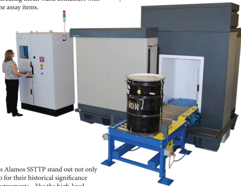
Figure 11. The high efficiency passive neutron counter (HENC) system is a passive neutron coincidence counter designed to assay 55 gallon drums of nuclear waste. The add-a-source technique can be used with the HENC to correct for measurement uncertainty owing to additional matrix elements in the waste (e.g., concrete, steel, glass, plastic, and paper). Credit: Mirion Technologies.
