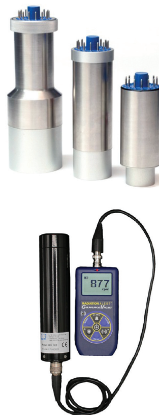
Figure 2. Inorganic scintillators emit light when exposed to ionizing radiation—one of the oldest known techniques for detecting radiation. Credit: CAEN SyS (caensys.com); S.E. International, Inc (seintl.com).
