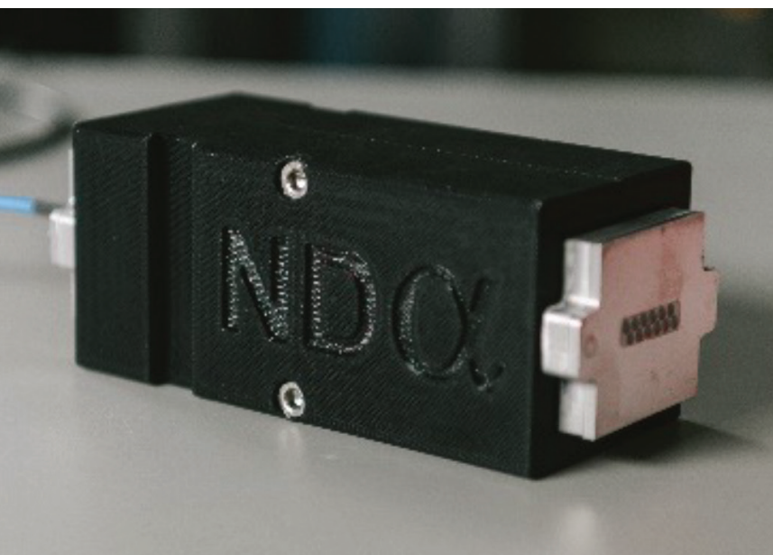
Figure 1. The portable ND-Alpha instrument, designed to use as a point-and-shoot detector with no sample preparation needed.
