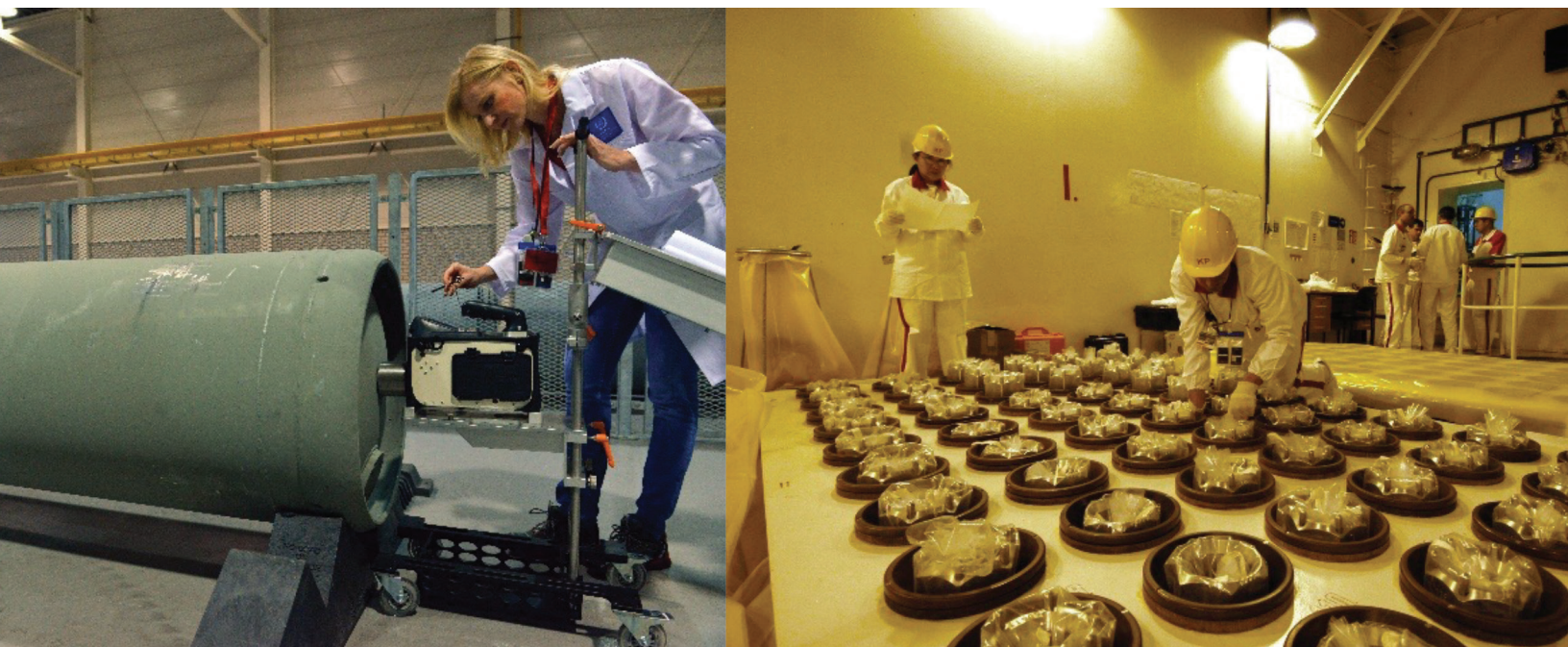
Figure 1. Left: An IAEA inspector uses an HPGe gamma detector to measure enriched uranium at URENCO in the Netherlands. Right: IAEA inspectors doing a physical inventory of nuclear fuel assemblies stored on a fresh fuel rack at Slovakia's Mochovce nuclear power plant. Credit: IAEA/Dean Calma.
