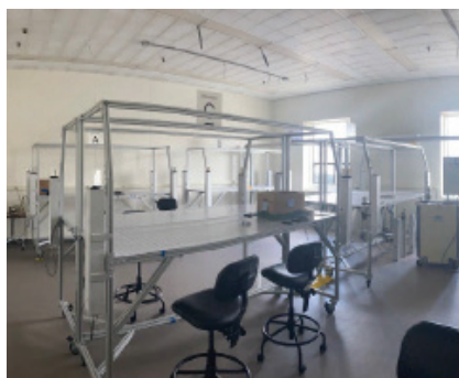
Figure 5. To optimize the distributed sensor network of the DBCM system, researchers developed a testbed consisting of four mock gloveboxes, each equipped with helium-3 detectors at all four corners. This setup enables evaluation of the network's capability to monitor nuclear material under various glovebox configurations.
