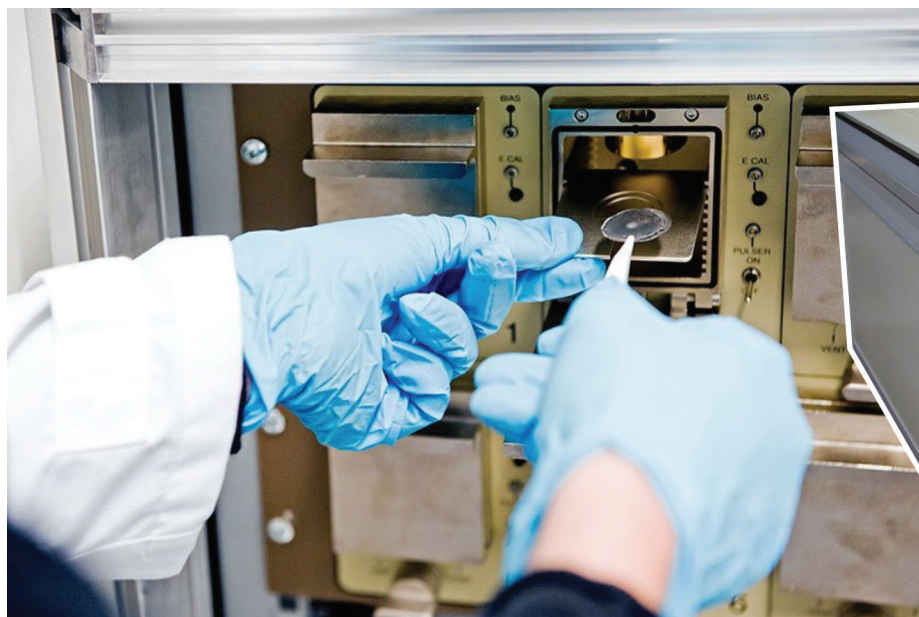
Figure 2. Example of a traditional benchtop alpha spectrometer, which works by measuring the alpha emission spectrum from a prepared sample placed in a vacuum chamber. Credit: Mirion Technologies, Inc.; physicsopenlab.org .
