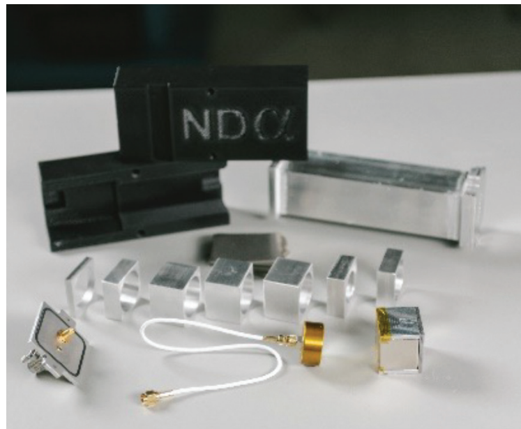
Figure 1. The portable ND-Alpha instrument, designed to use as a point-and-shoot detector with no sample preparation needed.
