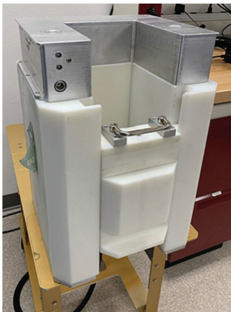
Figure 10. Uranium neutron coincidence collar (UNCL-II) design. It consists of three polyethylene sides that contain helium-3 detectors and a fourth side (at front) that contains an americium-241/lithium source. This is the primary NDA system used by IAEA inspectors to verify uranium content in light-water reactor fresh fuel assemblies. Credit: PANDA manual.
