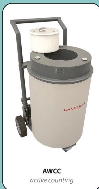
Figure 9. Left: JCC-31 high level neutron coincidence counter (HLNCC); Right: JCC-51 active well coincidence counter (AWCC). The HLNCC is an example of a passive neutron counter and is the standard instrument for assaying plutonium content up to a few kilograms. The AWCC meanwhile uses active neutron interrogation with an americium-241/lithium source of neutrons, located immediately beneath the cavity, which is useful for assays of uranium-235. Both these instruments were developed through a technology transfer from Los Alamos National Laboratory. Credit: Mirion Technologies.
