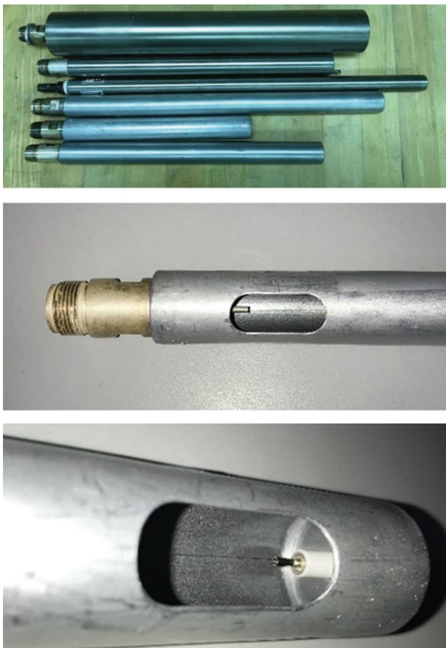
Figure 8. Various sizes of gas-filled neutron detectors (top) and cut-out views of a typical helium-3 detector tube (middle and bottom). Credit: Geist, Santi, and Swinhoe, “Nondestructive Assay of Nuclear Materials for Safeguards and Security,” 2024 (known as the PANDA manual).
