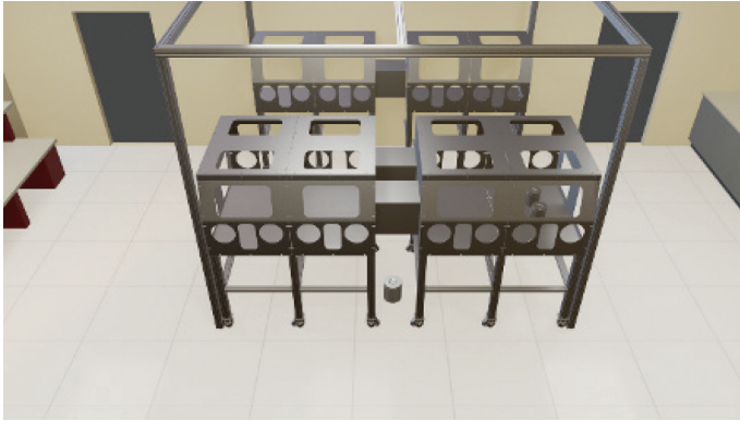
Figure 5. The 3D visualization tool supports real-time RFID tracking, allowing users to visualize asset movement through rooms. Left: Mock-up gloveboxes rendered with the 3D visualization tool for asset localization tracking. Right: The 3D visualization tool shows the position of a nuclear material container as it moves through the aisle between different mock-up gloveboxes.
