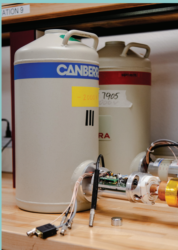
Figure 7. A high purity germanium (HPGe) detector with its electronic components exposed, attached to a liquid nitrogen dewar for cooling to enable it to operate and detect radiation. This cooling process is crucial to reduce leakage current and noise, which would otherwise degrade the detector's energy resolution. The crystal of high purity germanium from a separate detector is visible on tabletop below; HPGe crystals are engineered single-crystal ingots, free of dislocations and defects, with exceptional purity levels (up to 13N or 99.9999999999%).
