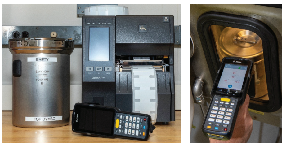
Figure 3. A LANL SAVY container fitted with RFID tag along with commercial Zebra reader and label printer, which has UHF RFID encoding capability. The SAVY-4000 is a container system developed by LANL for the safe storage of solid nuclear materials, first deployed in TA-55 in 2011.
