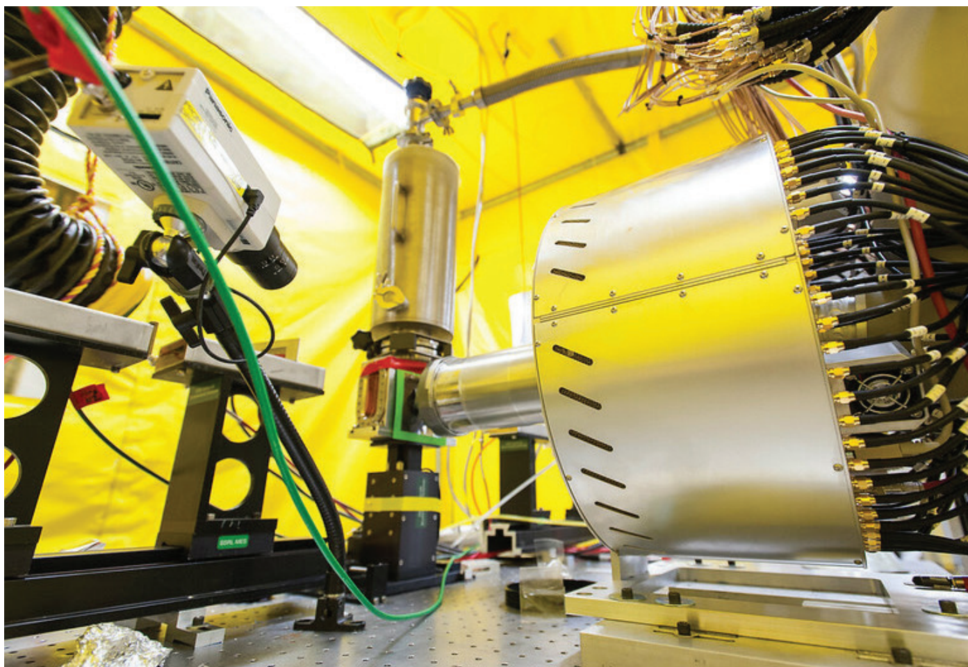
Beamline 11-2 at the Stanford Synchrotron Radiation Lightsource (SSRL) is a high-flux X-ray absorption spectroscopy (XAS) station dedicated to molecular biogeochemical and interface sciences. It is optimized for challenging XAS measurements on dilute or radioactive samples and interfaces. Credit: SSRL.
