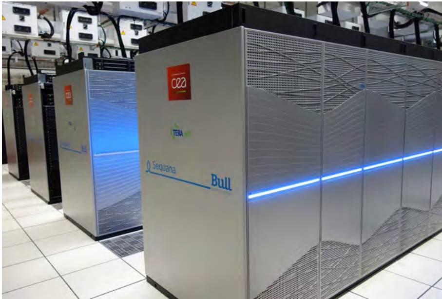
Figure 3. The Tera-1000 supercomputer. With 25 petaflops computing power it is the most powerful European general-purpose supercomputer in use. It was developed in 2018 at the CEA (French Alternative Energies and Atomic Energy Commission) center in Bruyères-le-Châtel (Île-de-France).
