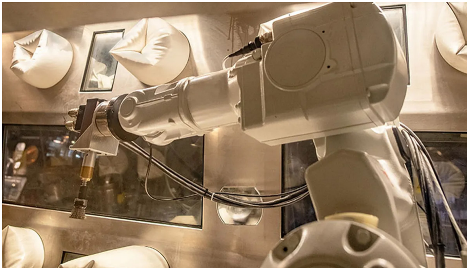
A robotic arm inside a demonstration glovebox, similar to those where plutonium parts for nuclear weapons are handled, can help reduce human radiation exposure.
