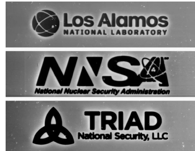
A suite of logos etched onto silicon by a focused ion beam. Each logo is just 100 microns across, roughly the same width as a human hair. Image Credit: Ben Morrow
