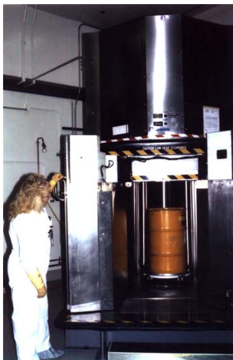
Fig. 5. Sandra Hildner opens the doors of the shuffler for 200-liter drums at the Los Alamos Plutonium Facility to reveal a 200-liter drum. This shuffler is used to measure pyrochemical salt residues. These salts have very high ^{241}\text{Am} levels that produce large \alpha, n rates that defeat passive coincidence methods. The shuffler can override this neutron background and achieve good measurement results.
