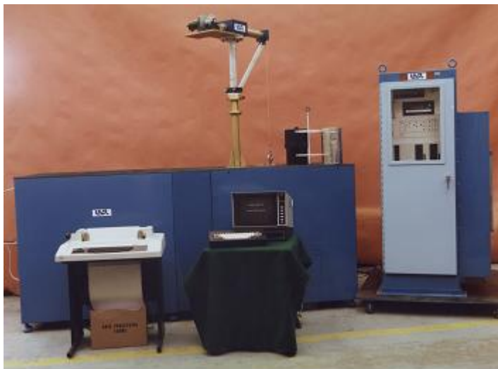
Fig. 2. The Uranium Scrap Shuffler had a hoist to raise and lower the heavy cans of scrap. A computer in an air-conditioned electronics rack was used to control the instrument and analyze the data.
